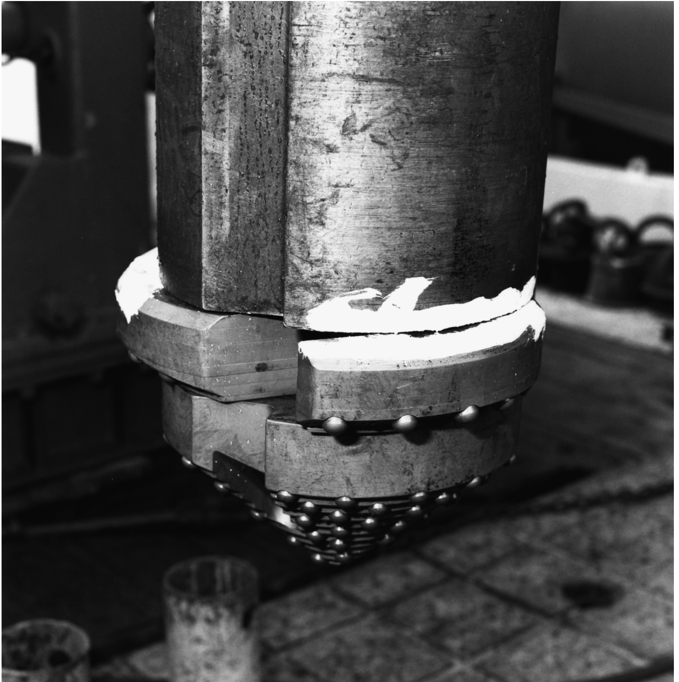
Figure F18. Holte concentric underreamer bit (before deployment).
