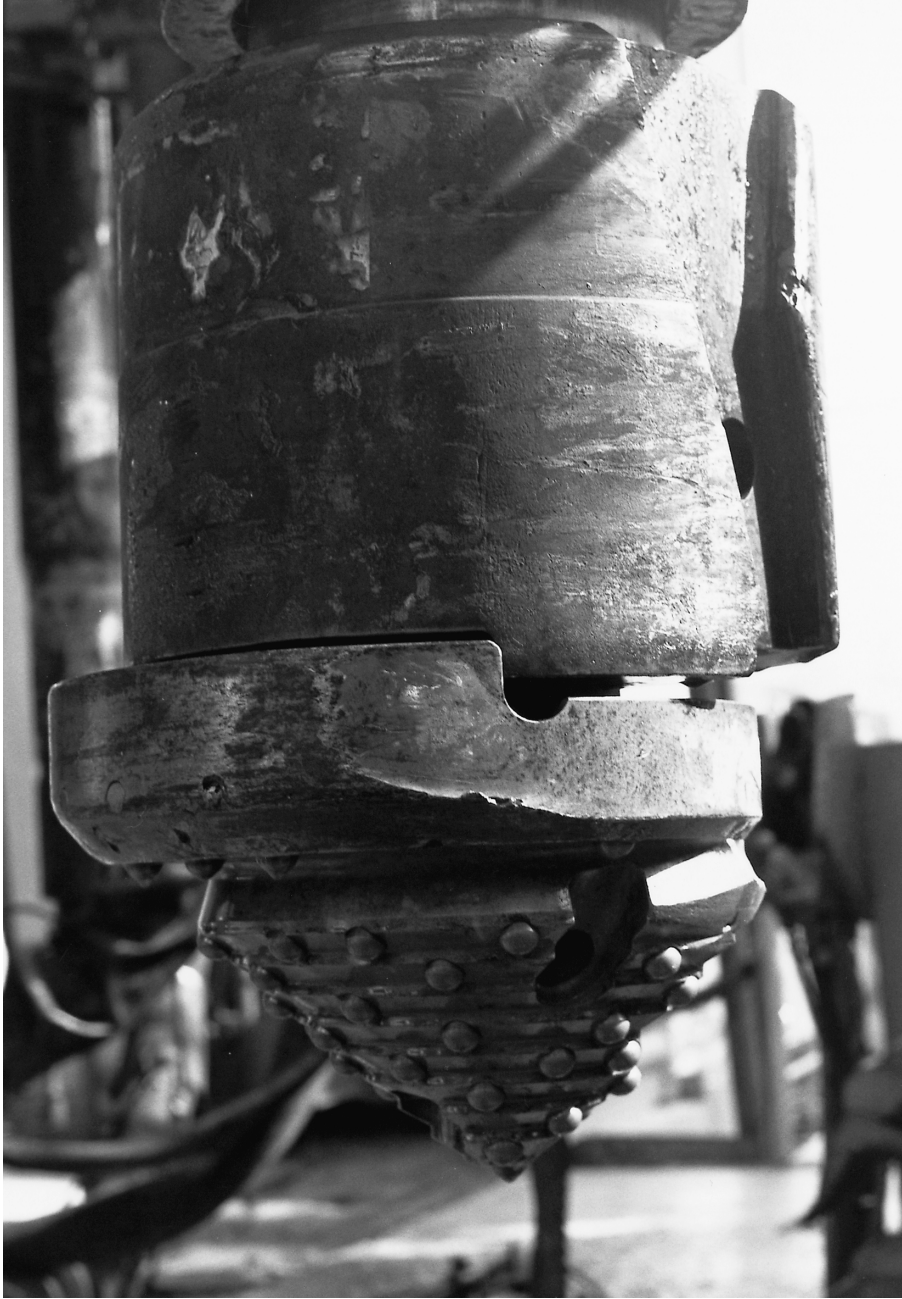
Figure F19. Holte eccentric underreamer bit.
