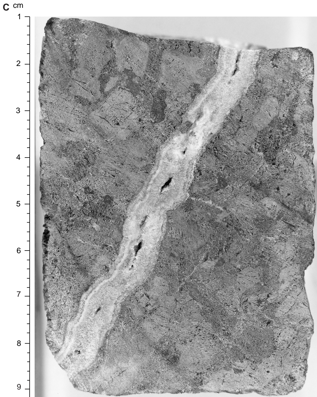
Figure F71 (continued). C. Close-up core photograph of smectite-clay veins within fractures in vuggy calcite veins in interval 179-1105A-30R-1, 1-9 cm.
