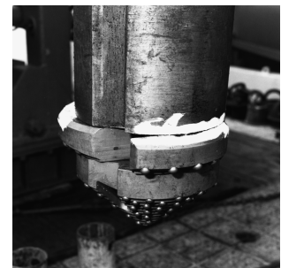
F18. Holte concentric underreamer bit, p. 90.
