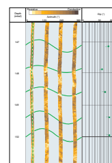
F65. Hole 1114A statically normalized FMS image and tadpole plot, upper log Unit L3, p. 114.
