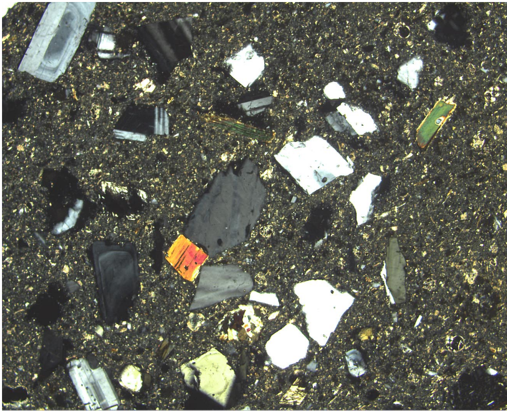
Figure F5. Digital photomicrograph (crossed nicols) of a silty claystone with common unaltered detrital grains of plagioclase, biotite, hornblende, and planktonic foraminifers. Note the zoned plagioclase (lower left) (interval 180-1115C-10R-1, 5–7 cm).
