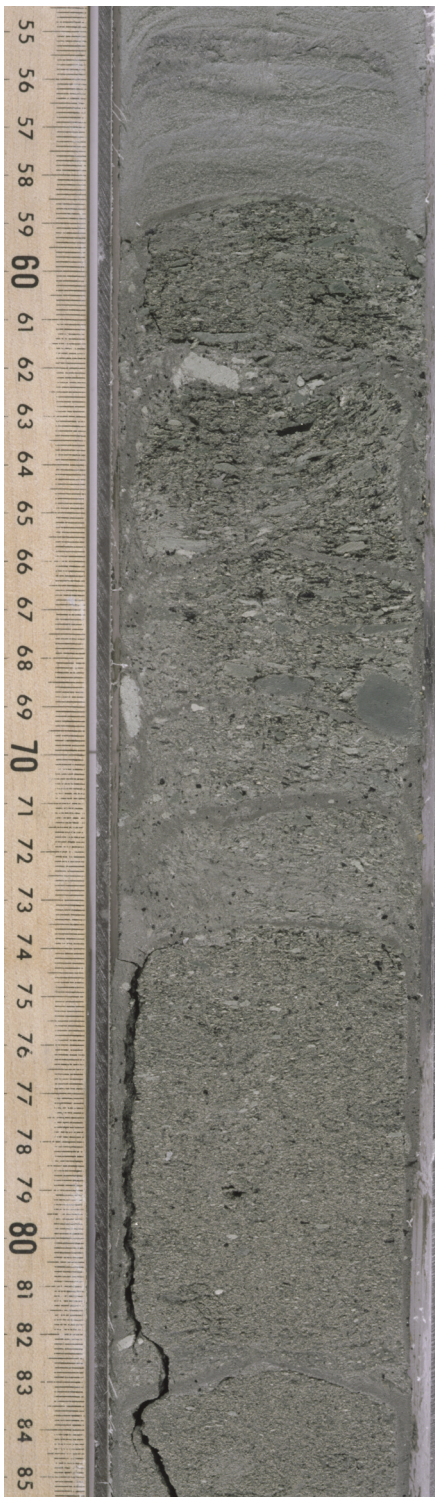
Figure F11. Reverse-graded debris-flow deposit in Subunit IIIB (interval 181-1122C-67X-1, 55–85 cm; 608.75–609.05 mbsf).
