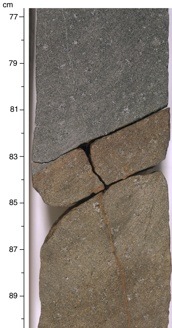
Figure F37. Close-up photograph of Sample 183-1140A-34R-3 (Piece 1, 77–90 cm). Sharp boundary between gray basalt and an oxidized orange-brown alteration halo related to the underlying contact with dolomitized chalk. The most intense coloration in this halo is at the boundary. The ~1-mm vein that cuts this boundary changes from light green clay to brown clay ( \pm iron oxyhydroxides).
