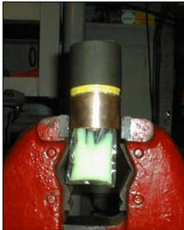
Figure F4. A. Spacer with a channel for the top of the Whirl-Pak bag containing the fluorescent microspheres. B. Bag containing 40 mL of the fluorescent microsphere suspension attached to the spacer. (Continued on next page.)
