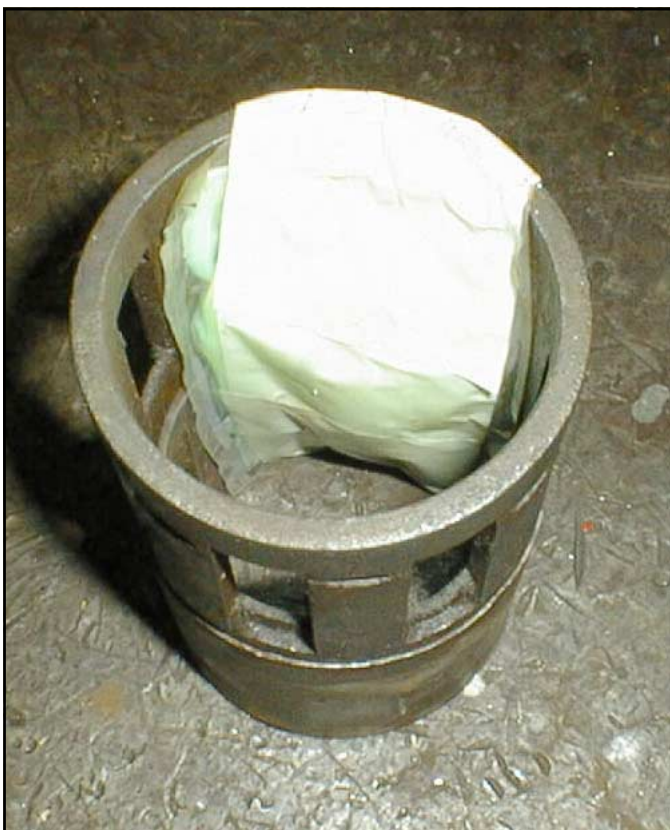
Figure F4 (continued). C. Bag containing microsphere suspension draped over the core-catcher body. D. The complete assembly for placing the microspheres in the core barrel. Top: petal flapper core catcher with metal sleeve. Middle: brass spacer with metal sleeve. Bottom: core-catcher body.
