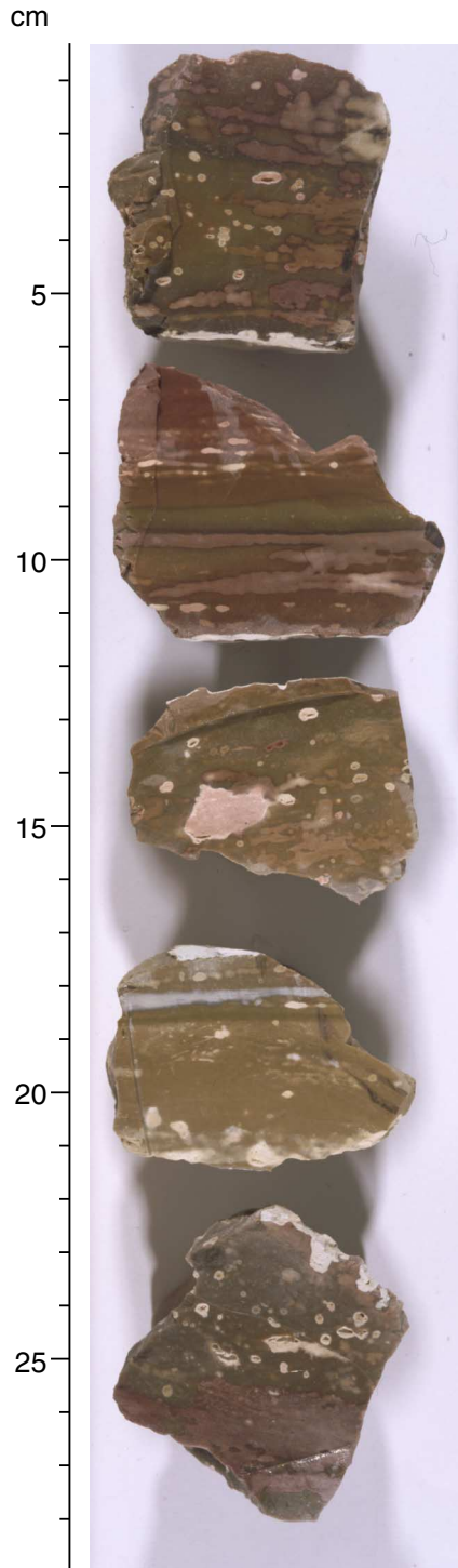
Figure F28. Chert pieces with “swiss cheese” type lenses of less indurated, partly calcareous material (interval 185-1149B-25R-1, 0–29 cm).
