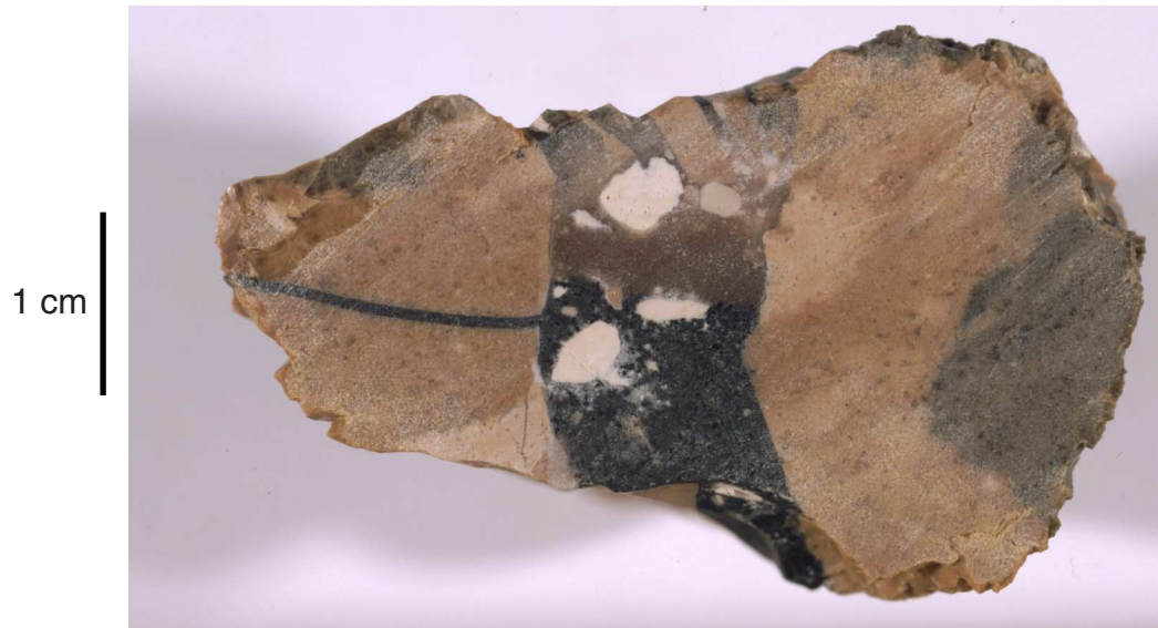
Figure F21. Pink chert with chalcedony-filled vein. Note light pink-colored lenses of porous porcelainite (interval 185-1149B-6R-1, 20–25 cm).
