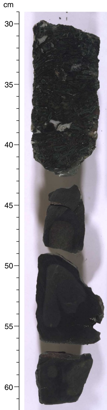
Figure F38. Hyaloclastite from Hole 1149D. Angular and elongate altered glassy shards in a green clay cement, with some carbonate present (interval 185-1149D-7R-1, 29–62 cm).
