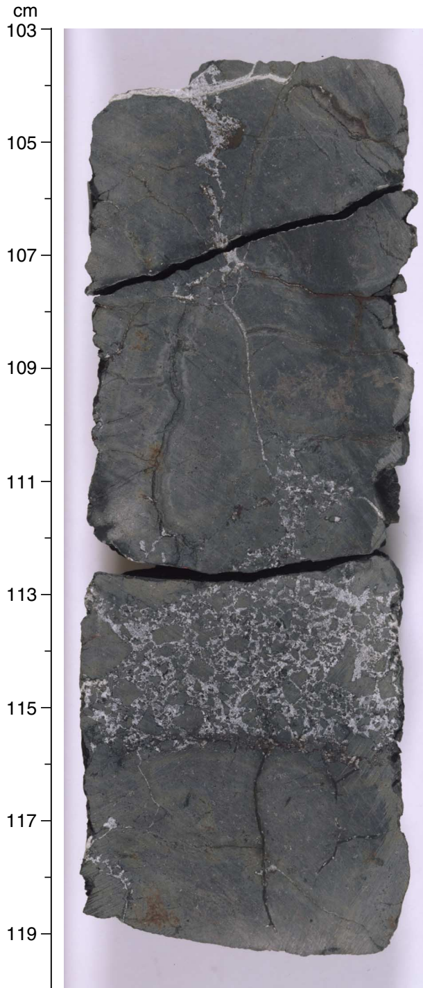
Figure F37. Brecciated basalt from Hole 1149D. Breccia consists of angular basalt pieces and medium-grained calcite cement. However, this interval also contains a microbreccia with basalt clasts all <1 cm in diameter (interval 185-1149D-11R-2, 103–119 cm).
