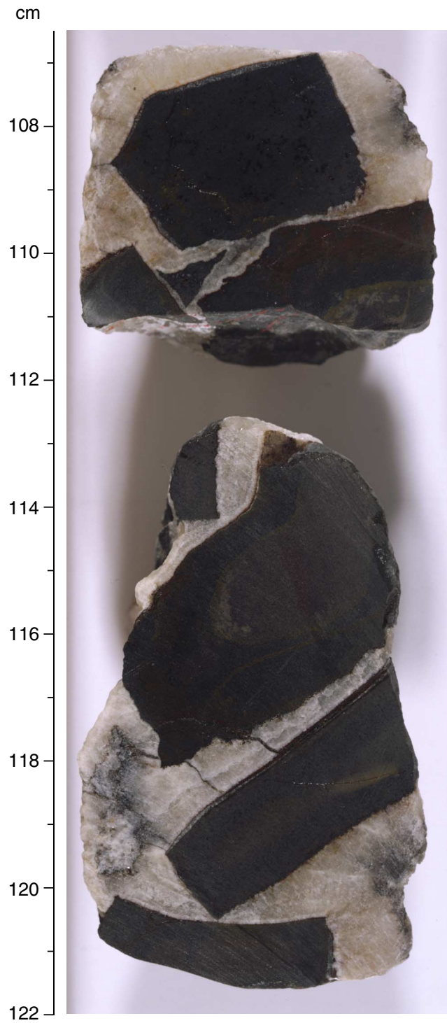
Figure F36. Brecciated basalt from Hole 1149C. The breccia consists of angular basalt pieces and medium-grained calcite cement (interval 185-1149C-10R-1, 107–121 cm).
