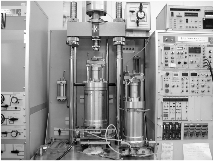
Figure F2. Triaxial compression instrument for consolidation and permeability testing.
