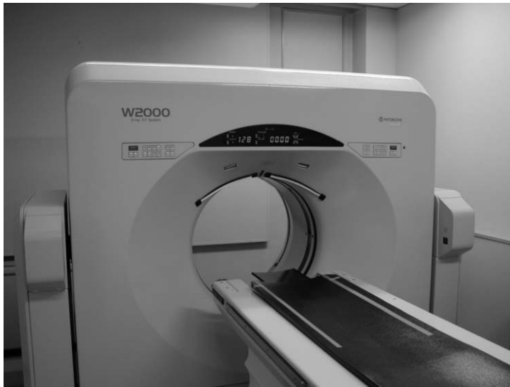
Figure F4. A. Photograph of the medical X-ray CT scanner W2000. B. Schematic of slice imaging of an X-ray CT. C. Thickness of each slice = 1 mm.
