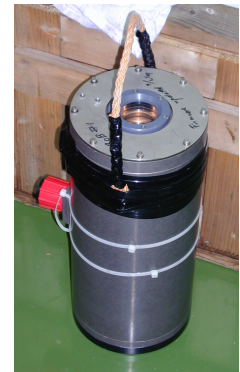
F17. Photograph of the BOB communication link between ROV and NEREID, p. 39.
