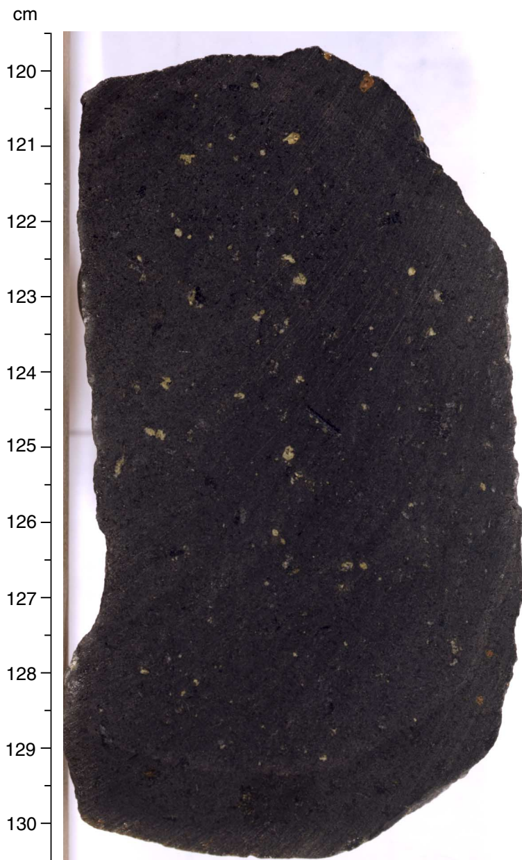
Figure F10. Photograph of interval 187-1154A-3R-1, 120–130 cm, showing light gray, moderately plagioclase-olivine phyric pillow basalt, typical of that recovered throughout Hole 1154A. Black irregular patches were formed by the plucking of altered groundmass from the cut surface.
