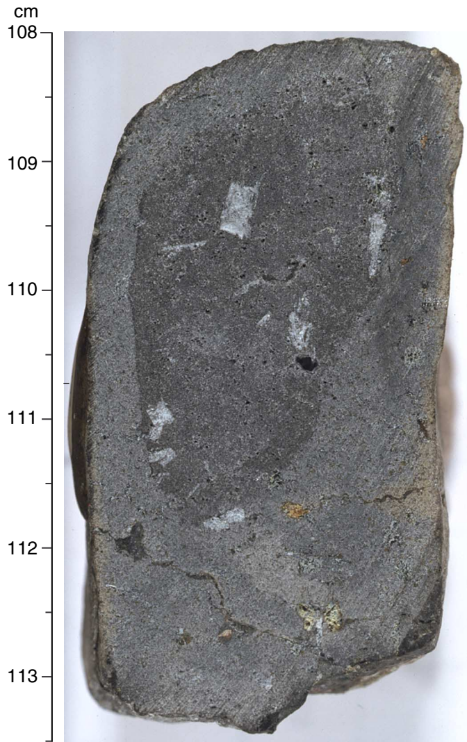
Figure F13. Photograph of interval 187-1152B-5R-1, 107–114 cm, showing large euhedral plagioclase phenocrysts in a sparsely plagioclase-olivine phyric basalt.
