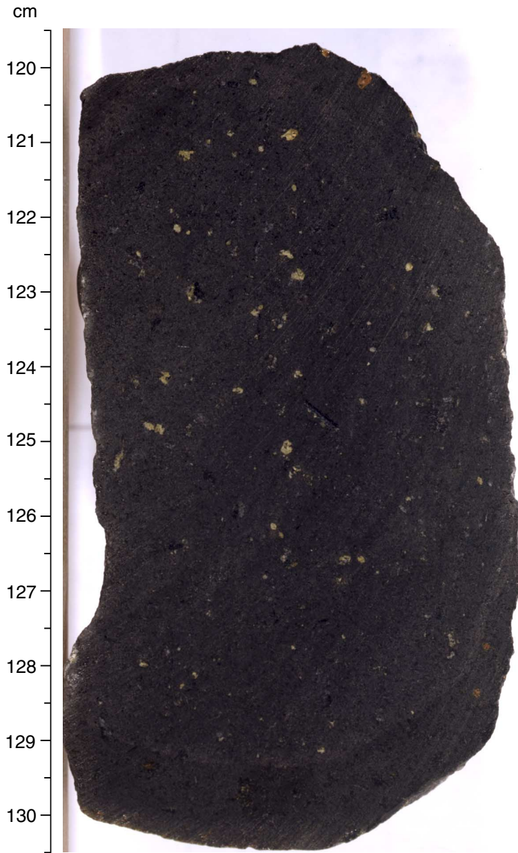
Figure F1. Photograph of interval 187-1154A-3R-1, 120–130 cm, showing light gray, moderately plagioclase-olivine phyric pillow basalt, typical of that recovered throughout Hole 1154A. Areas of altered groundmass plucked from the cut surface appear as black irregular patches.
