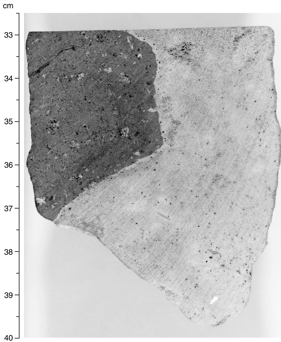
Figure F5. Photograph of interval 187-1157A-2R-1, 33–40 cm, showing calcarenite sediment partially enclosing a plagioclase-olivine phyric basalt clast.
