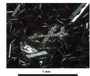
5 mm (e.g., Section 187-1163A-5R-1 [Piece 3]) before the more crystalline interior is reached. The unit contains ~2% spherical vesicles, on average 0.3 mm in diameter, with variable filling (see “Alteration,” p. 4) and ~3% miarolitic cavities (as large as 0.8 mm across) with euhedral elongate clinopyroxene (as large as 0.1 mm).
