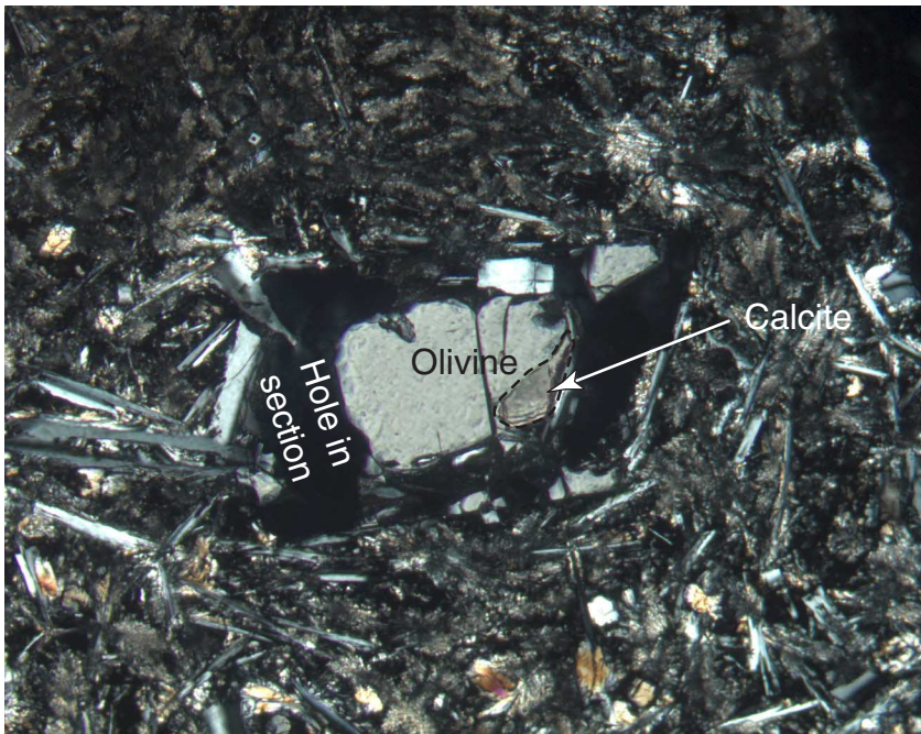
Figure F22. Photomicrograph, with crossed polars, of Sample 187-1164A-4R-1, 22–24 cm (see “ Site 1164 Thin Sections ,” p. 21), showing an olivine phenocryst partially replaced by calcite. Most calcite has been lost during sample preparation.
