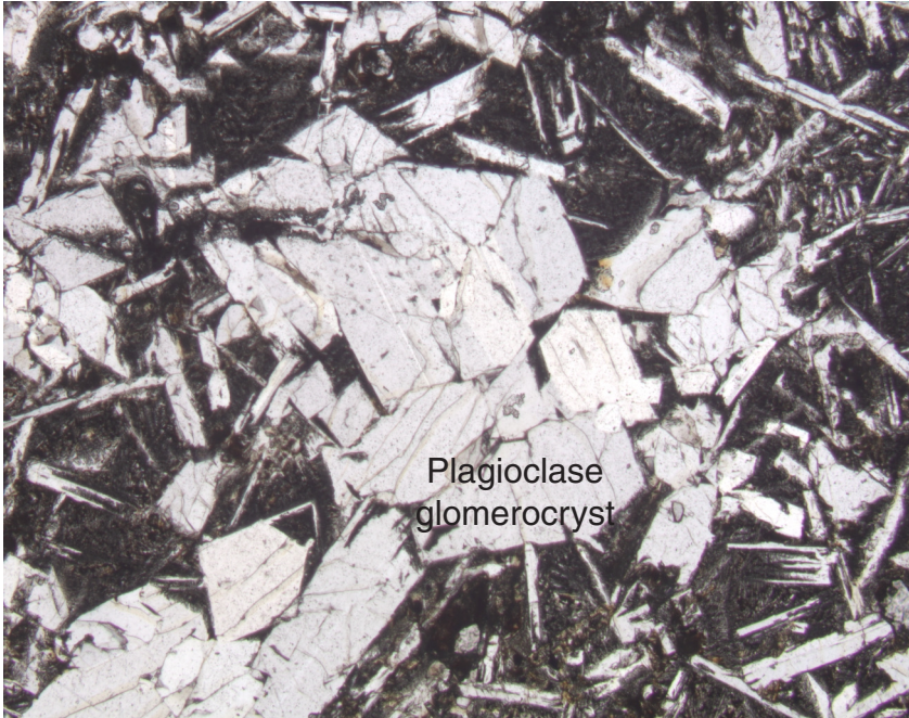
Figure F12. Photomicrograph of Sample 187-1164B-5R-1, 100–104 cm (see “Site 1164 Thin Sections,” p. 25), showing tightly clustered tabular plagioclase forming a glomerocryst.
