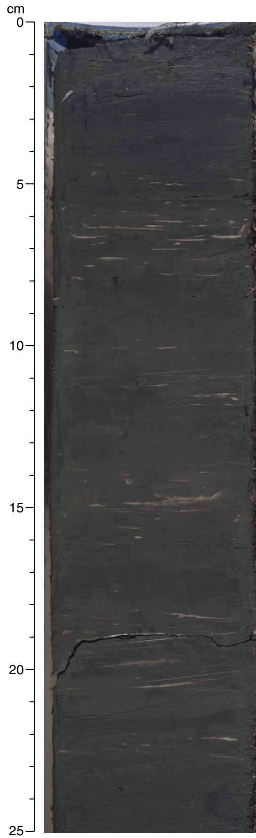
Figure F12. Facies II-3 clay with silt laminae (interval 188-1167A-25X-7, 0–25 cm). Note the cross-bedding of clays.
