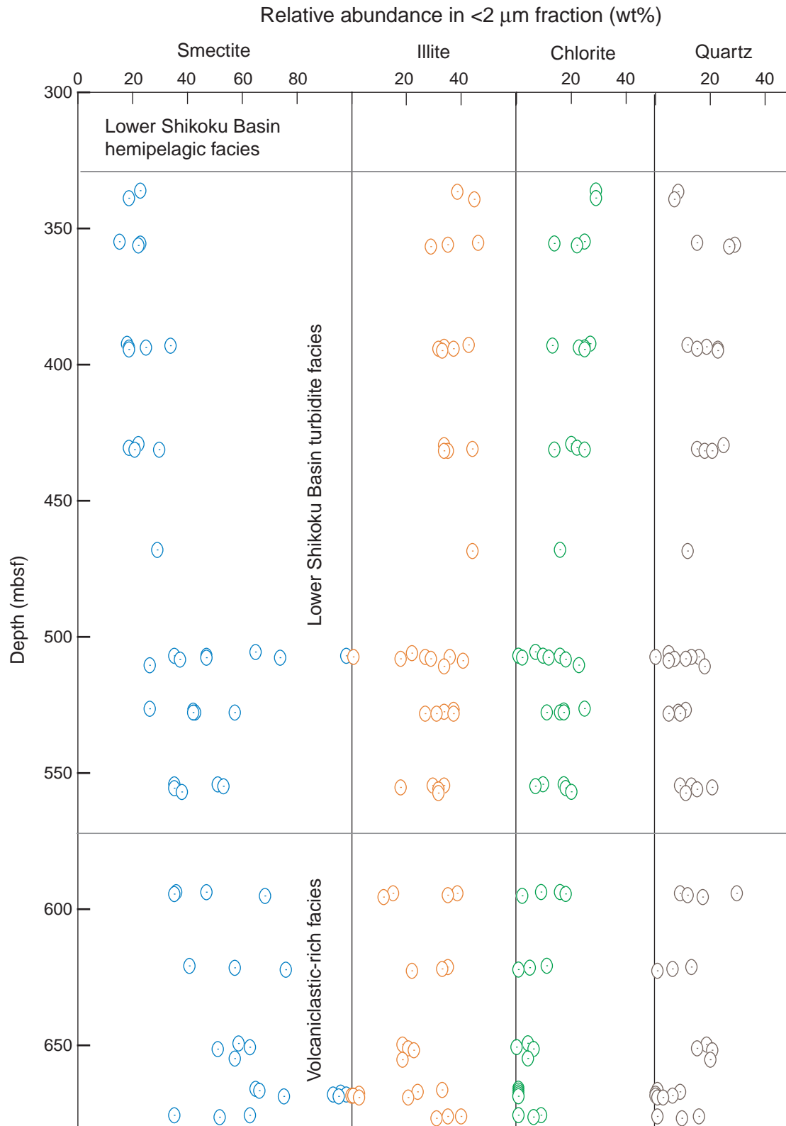
Figure F7. Results of X-ray diffraction analysis of oriented clay-sized aggregates from Site 297 of the Deep Sea Drilling Project. Data are tabulated in Table T8, p. 26. See Figure F1, p. 9, for location and Figure F6, p. 15, for stratigraphic column. Values of relative abundance (in weight percent) are based on the SVD (singular value decomposition) method using normalization factors shown in Table T4, p. 22.
