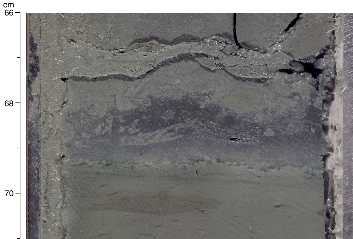
Figure F14. Bioturbated silty claystone and interbedded siliceous claystone from Unit III (interval 190-1173A-57X-4, 66–71 cm).
