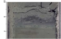
F8. Bioturbated silty claystone and interbedded siliceous claystone from Unit III, p. 45.
