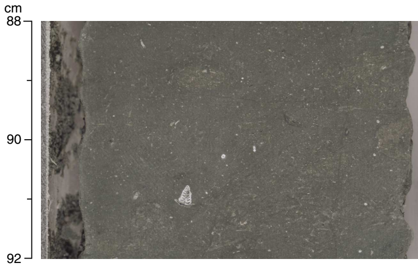
Figure F6. Silty claystone with foraminifers from the lower Shikoku Basin facies (interval 190-1174B-62R-3, 88–92 cm).
