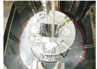
**F9.** Snapshot showing the PAT landed properly on top of the Hole 1179E reentry cone, p. 30.
