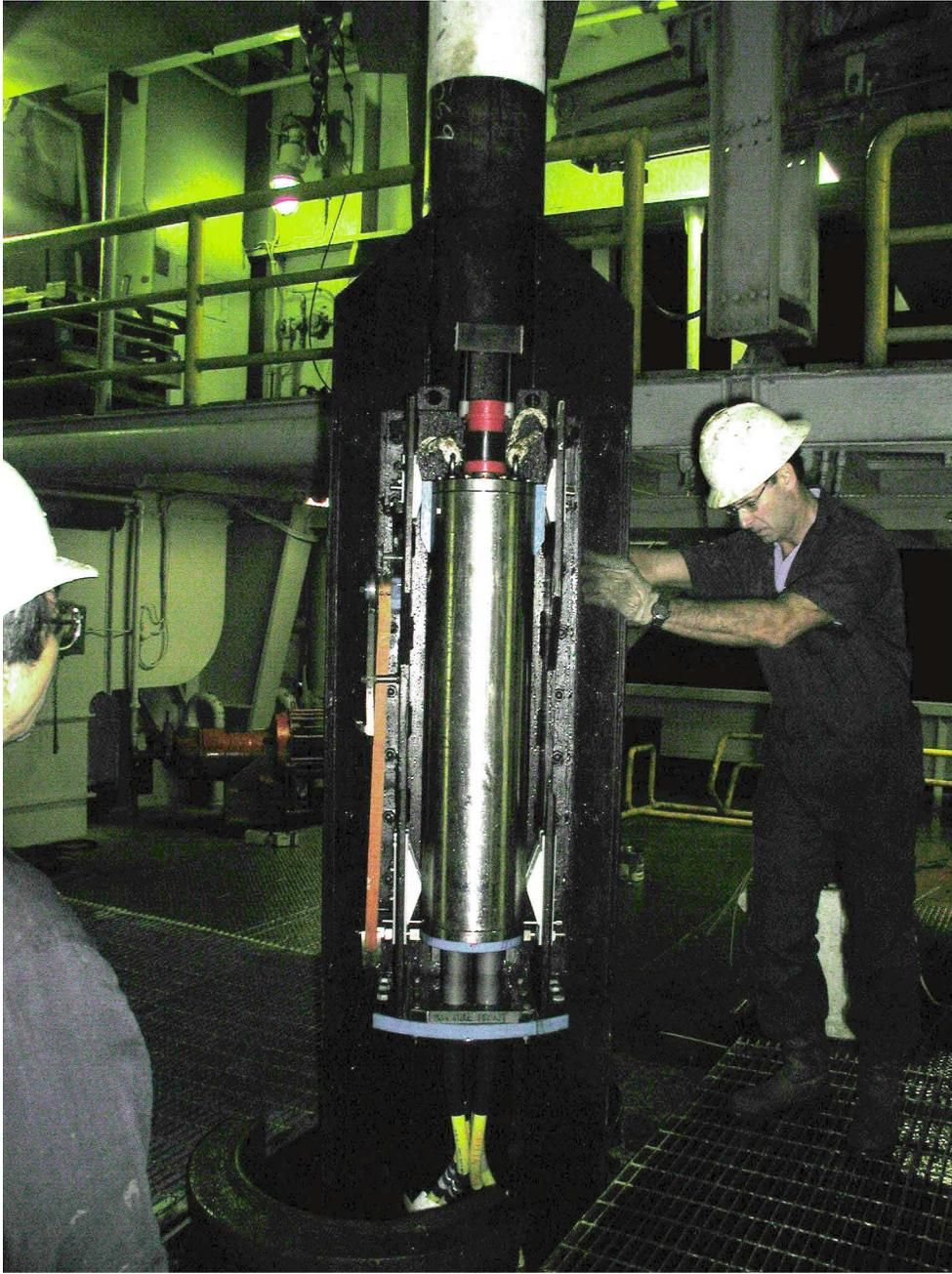
**Figure F8.** Power access terminal (PAT) battery frame being lowered through the moonpool. The PAT was hung on the logging line by a bridle assembly consisting of wire cables, nylon straps, three glass ball floats, and a redundant acoustic release.
