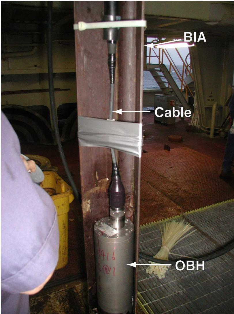
**Figure F9.** Installation of the borehole instrument assembly (BIA) in the moonpool area. After connecting the cables to the ocean borehole seismometer (OBH) sensors, cables were tied to the BIA with plastic tie wraps and duct tape.
