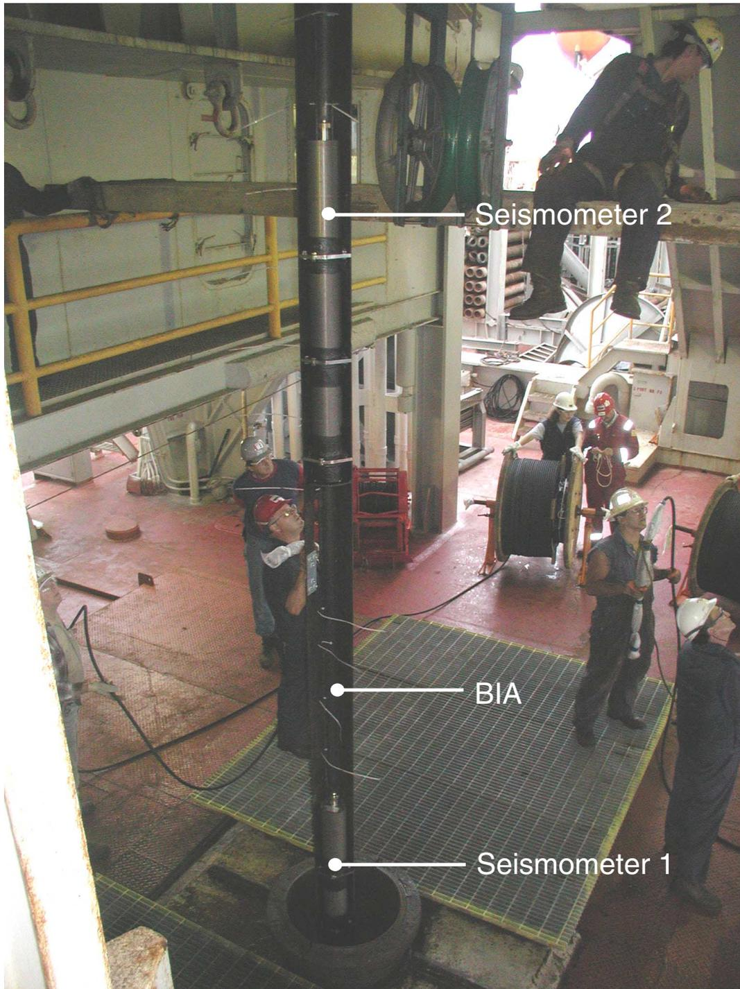
**Figure F6.** Appearance of the borehole instrument assembly (BIA). The BIA consists of a frame pipe and two blades. Its shape looks like a bottom of a ship. Two ocean borehole seismometer (OBH) sensors are emplaced on the BIA.
