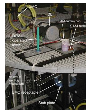
the mated position of the SAM-191 and the other at the released position. By the use of the locking positions, an ROV can easily replace the SAM-191 recorder.
