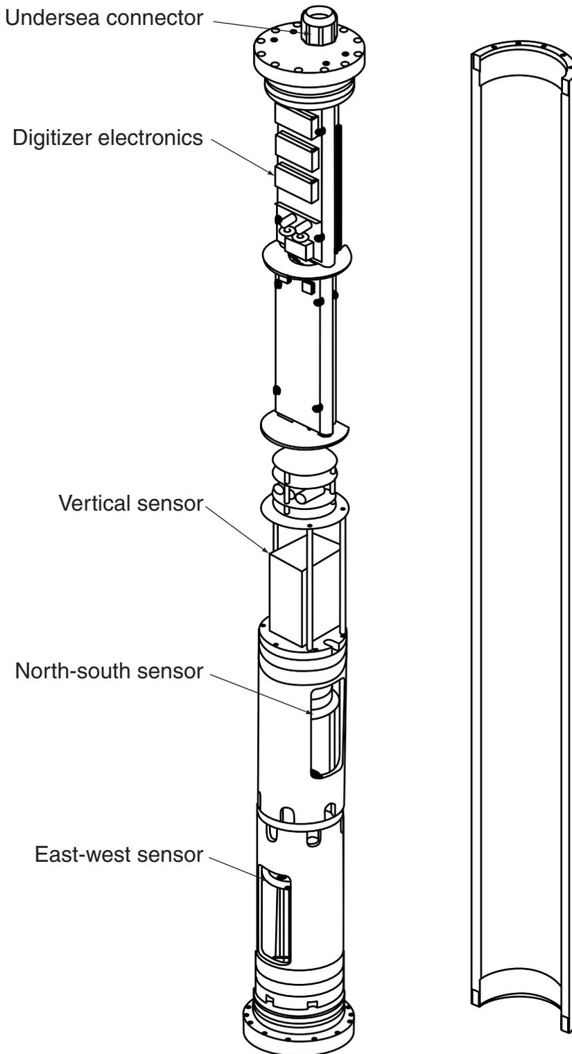
**Figure F13.** Cutaway drawing of the CMG-1T vertical sensor. The unit that appears in the drawing is mounted on a brass base, which holds the electronics circuit boards as well.
