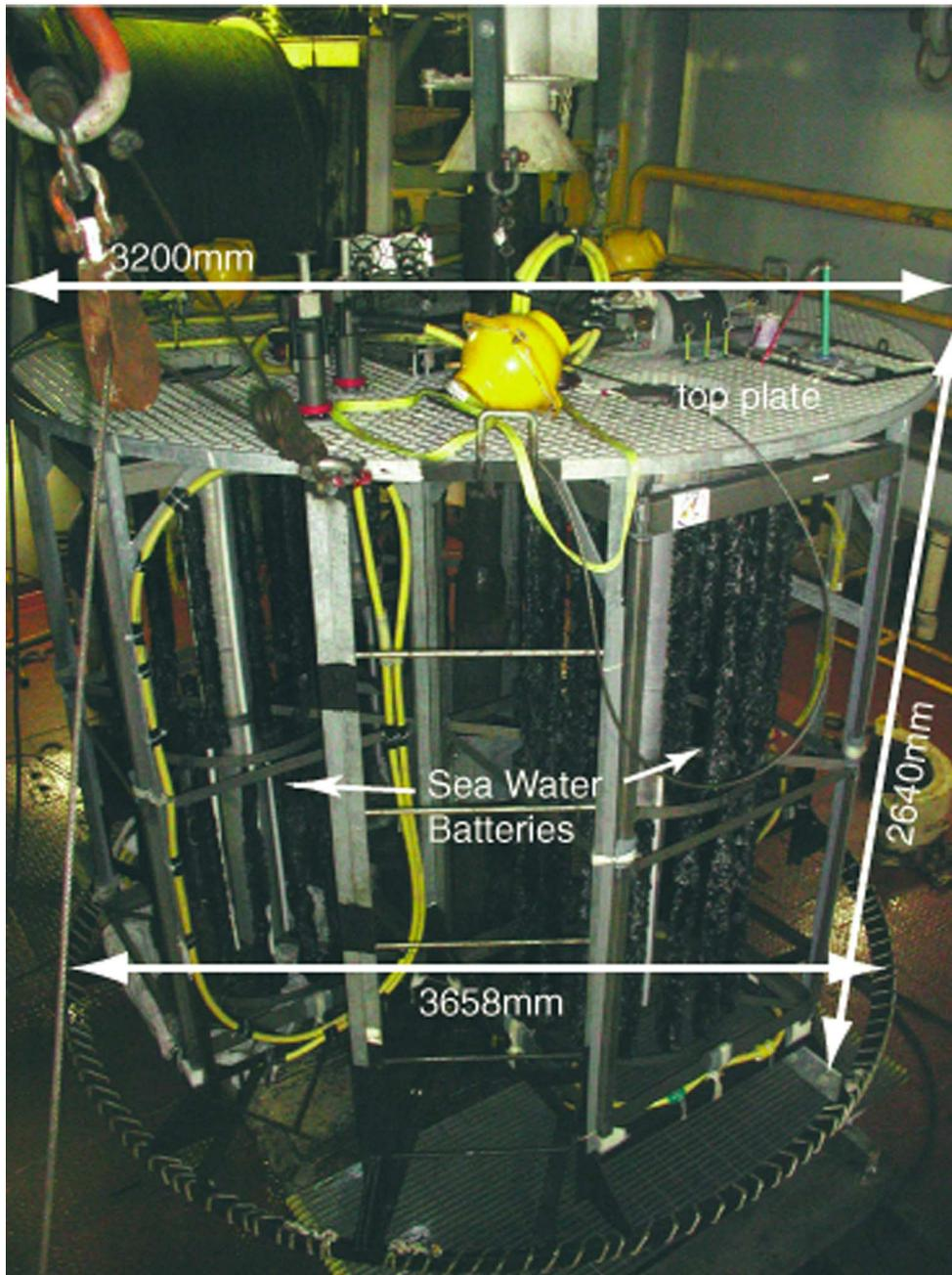
Figure F28. Photograph of the recorder frame of the storage acquisition module (SAM) with a SAM dummy cap. The recorder frame has a mechanism ejecting the SAM-191 by pulling the remotely operated vehicle (ROV)-operated lever. UMC = underwater mateable connector, DL = data logger.
