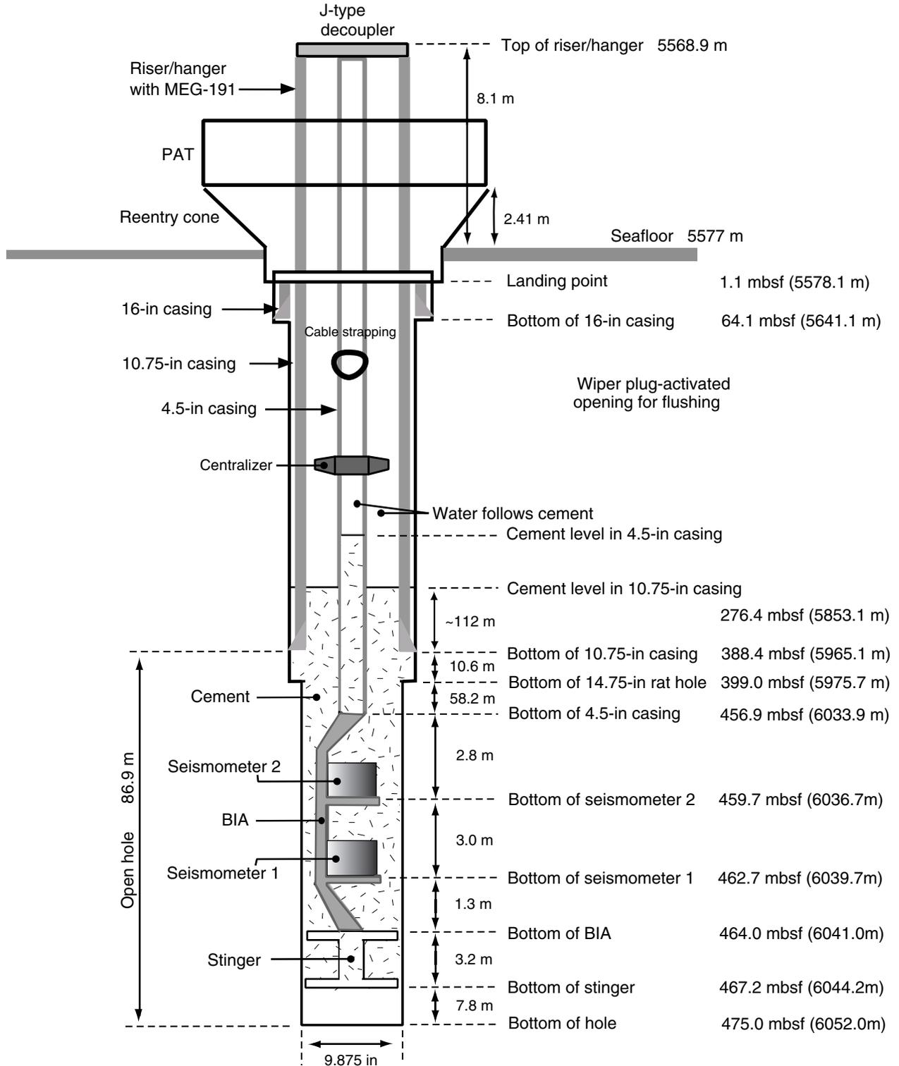
Figure F4. Cable strappings and centralizer.
