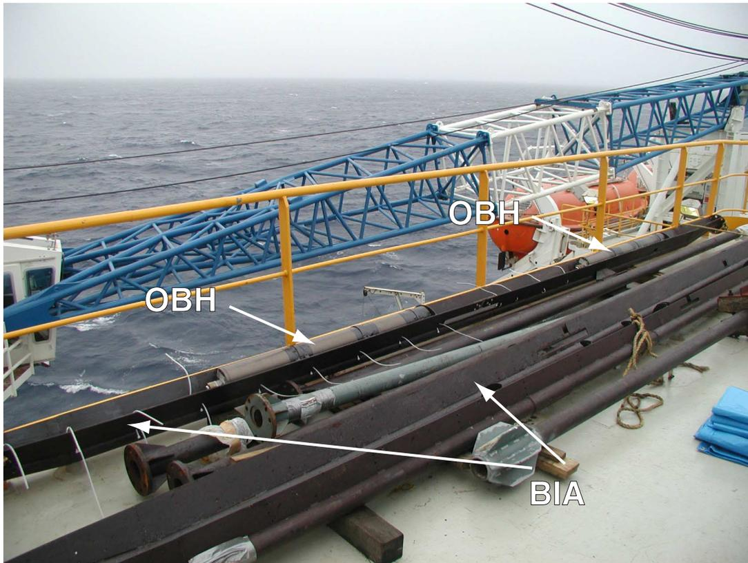
**Figure F7.** An ocean borehole seismometer (OBH) sensor was emplaced on the borehole instrument assembly (BIA) within the area enclosed by two blades.
