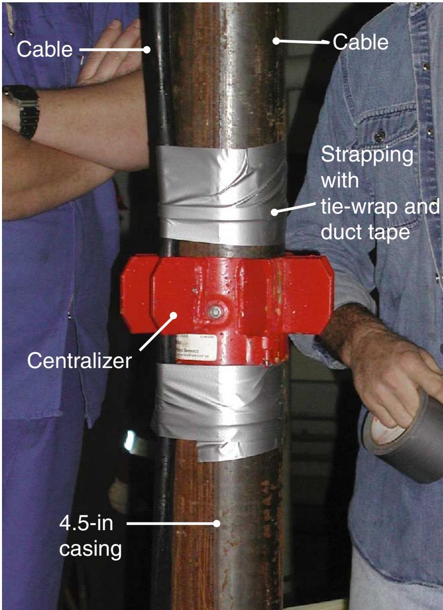
Figure F5. Instrument placement. Note that the seismometers are not electrically in contact with the borehole instrument assembly (BIA).
