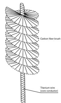
ply to the cathode. The oxygen supply rate is proportional to the oxygen concentration in the seawater and the speed of circulation. In order to produce the designed output of 6 W for each cell, a minimum circulation of 20 mm/s, an oxygen concentration of 3 ppm, and a salinity of 20‰ is required. Because the cells have an open structure, the isolation between cells is low, which leads to large leakage currents in serially connected cells. Thus, the cells are connected in parallel.
