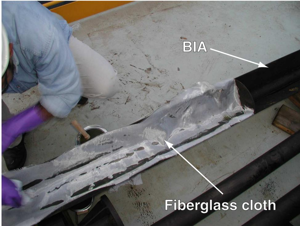
Figure F11. Fiberglass cloth was glued over surfaces of the borehole instrument assembly (BIA) where the ocean borehole seismometer sensors were affixed.
