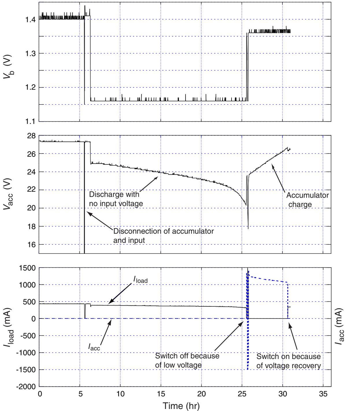
Figure F26. Records from the power control system during the final equipment test. The data were stored in the data logger. During this test, the low-voltage, high-current DC power supply was used in place of the SWB-1200 cells. SAM = storage acquisition module, MEG = multiple-access expandable gateway, OBH = ocean borehole seismometer.
