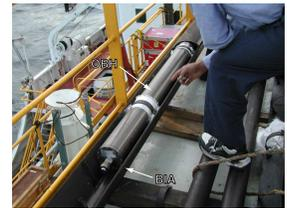
F8. Cable connections to the OBH during BIA installation, p. 29.
