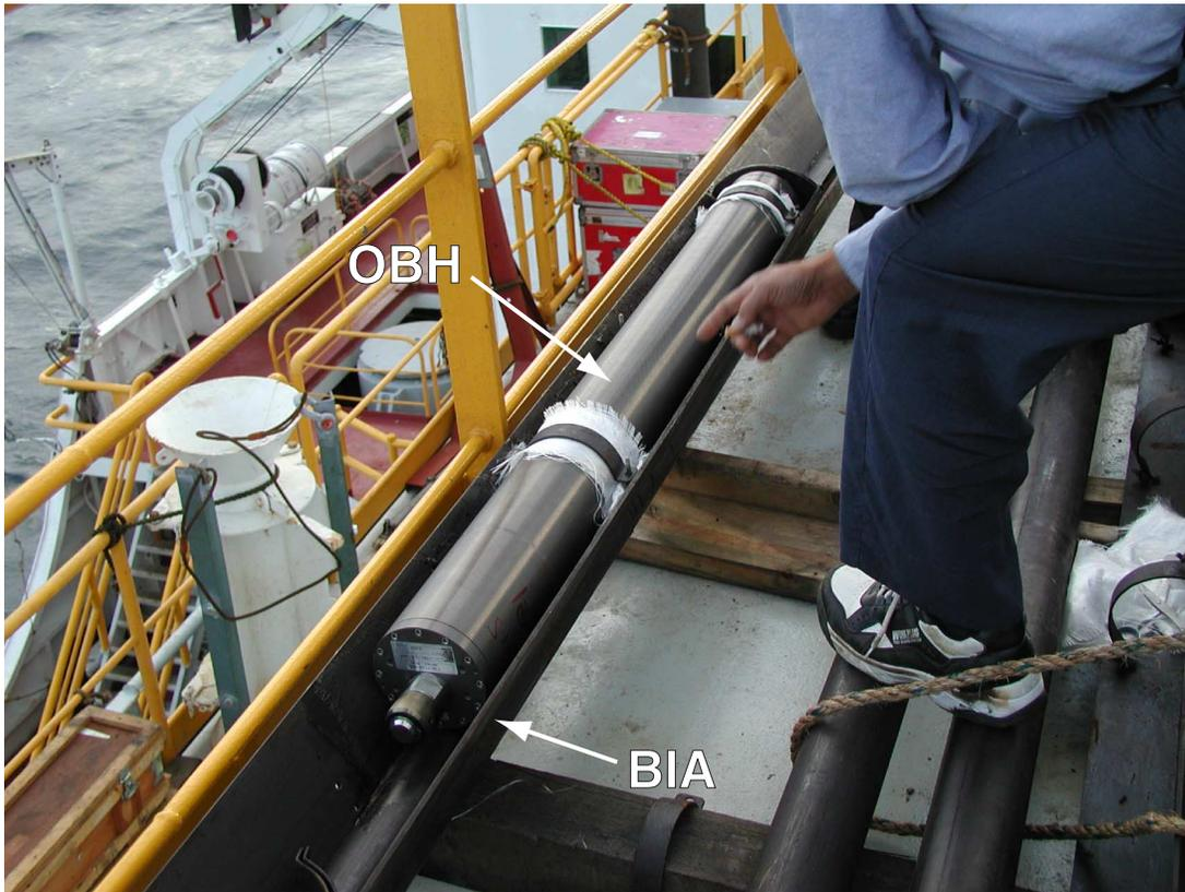
Figure F8. Installation of the borehole instrumentation assembly (BIA) in the moonpool area. After affixing the ocean borehole seismometer (OBH) sensors onto the BIA, the BIA was moved to the moonpool area for installation into the borehole. Cable connections to the OBH sensors were made.
