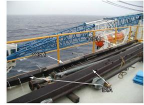
F7. An OBH sensor emplaced on the borehole instrument assembly, p. 28.
