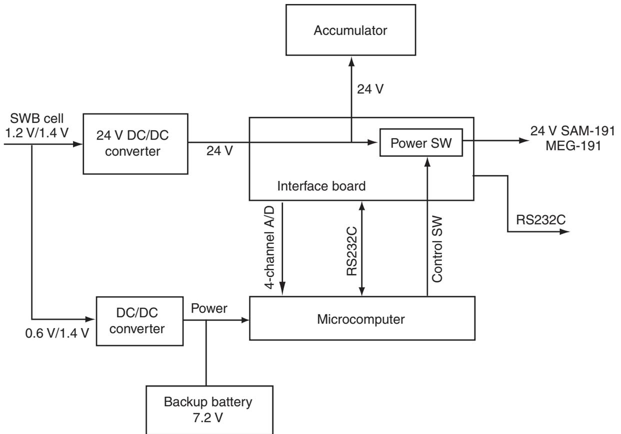
Figure F24. Voltages and currents measured by the power control system (PCS). The voltages are directly measured by an A/D converter on the PCS. The current is estimated by measurement of the voltage drop of a resistor with a small value, which is serially connected to the power line. SWB = seawater battery, Power SW = power switch.
