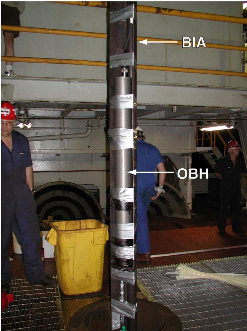
**Figure F10.** Insulation between the ocean borehole seismometer (OBH) sensors and the borehole instrument assembly (BIA) was made using fiberglass cloth.
