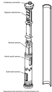
F13. Drawing of the CMG-1T vertical sensor, p. 34.
