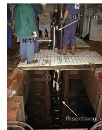
F75. MEG-191 on the riser/hanger, lowered into the moonpool, p. 127.
