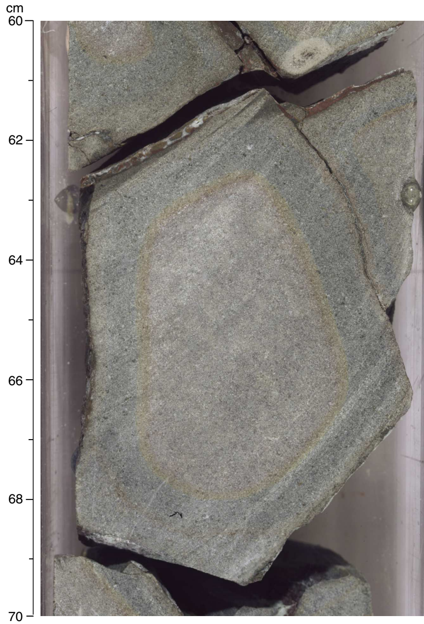
Figure F42. Close-up photograph of a liesegang structure in a basalt flow of Unit 1, formed by infiltration of fluids during alteration (interval 191-1179D-10R-1, 60–70 cm).
