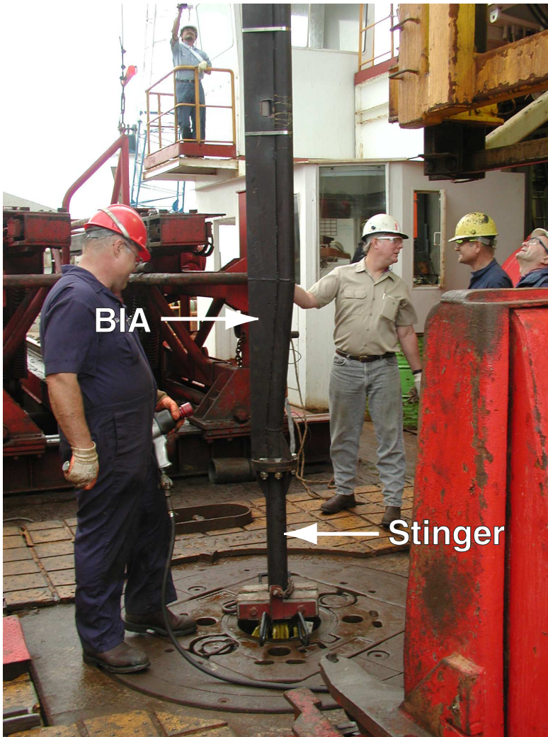
Figure F69. Stinger pipe jointed to the lower end of the borehole instrument assembly (BIA).
