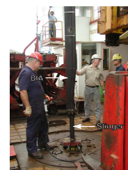
F69 . Stinger pipe jointed to the lower end of the borehole instrument assembly, p. 121.
