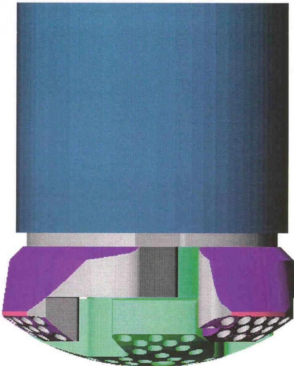
Figure F14. Side view of the dual cam underreamer bit with arms open. Tungsten carbide inserts are not illustrated.
