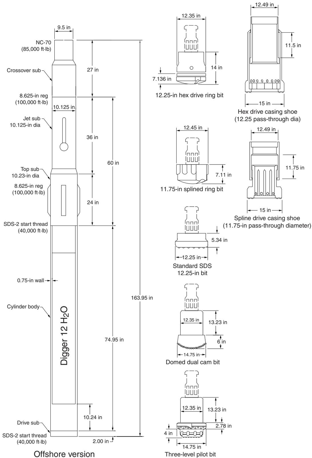
Figure F11. SDS modified top sub with centralizer pads (ODP style with 8.625-in reg box connection).
