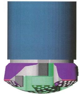
F14. Side view of the dual cam underreamer bit with arms open, p. 35.
