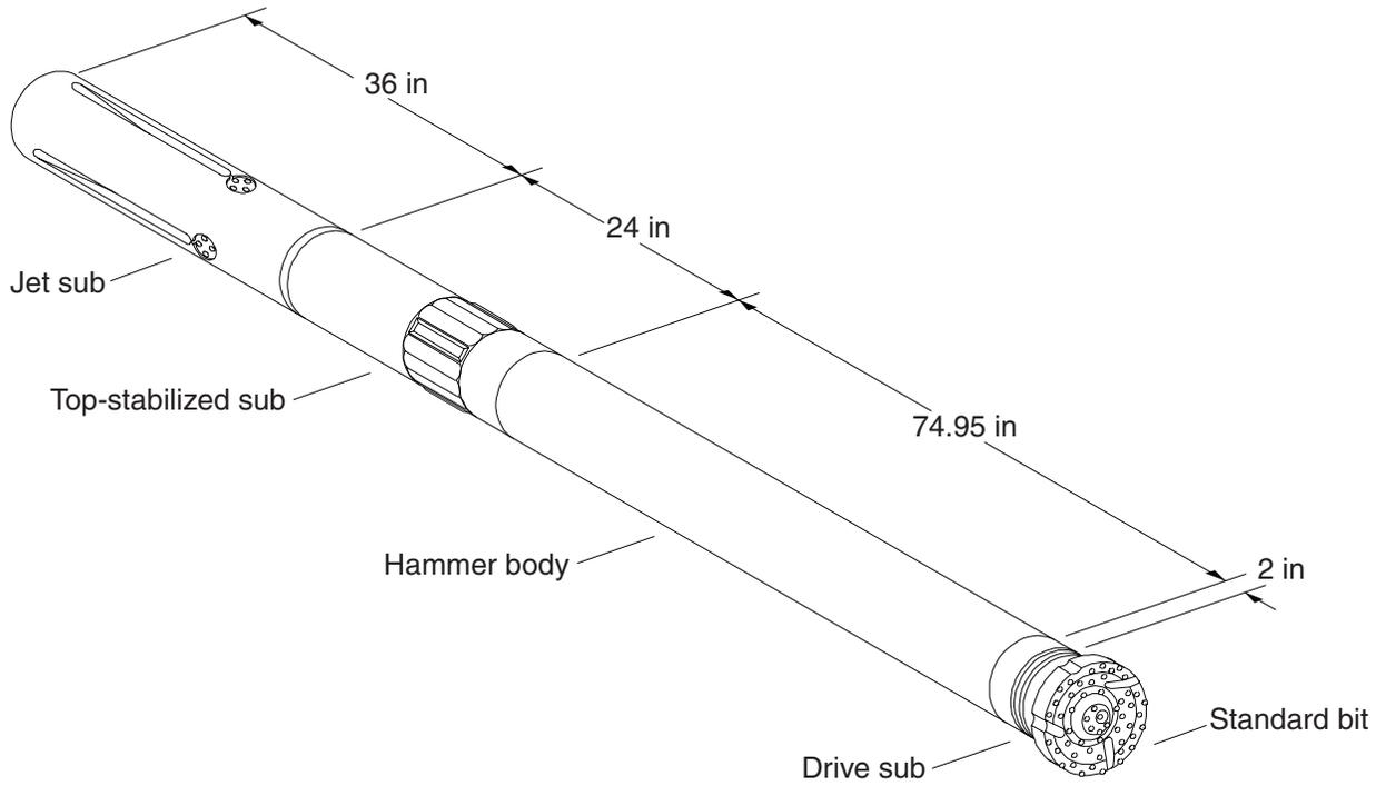
**Figure F10.** SDS 260 fluid hammer and test bit configurations. The make-up torque is shown in parenthesis.
