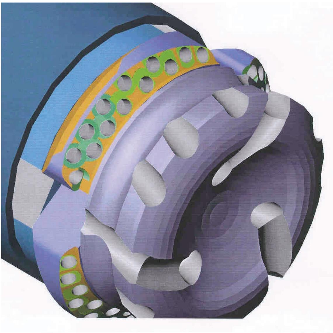
Figure F20. Pulsation sub. Both connections are NC-70. OD = outer diameter, ID = inner diameter.
