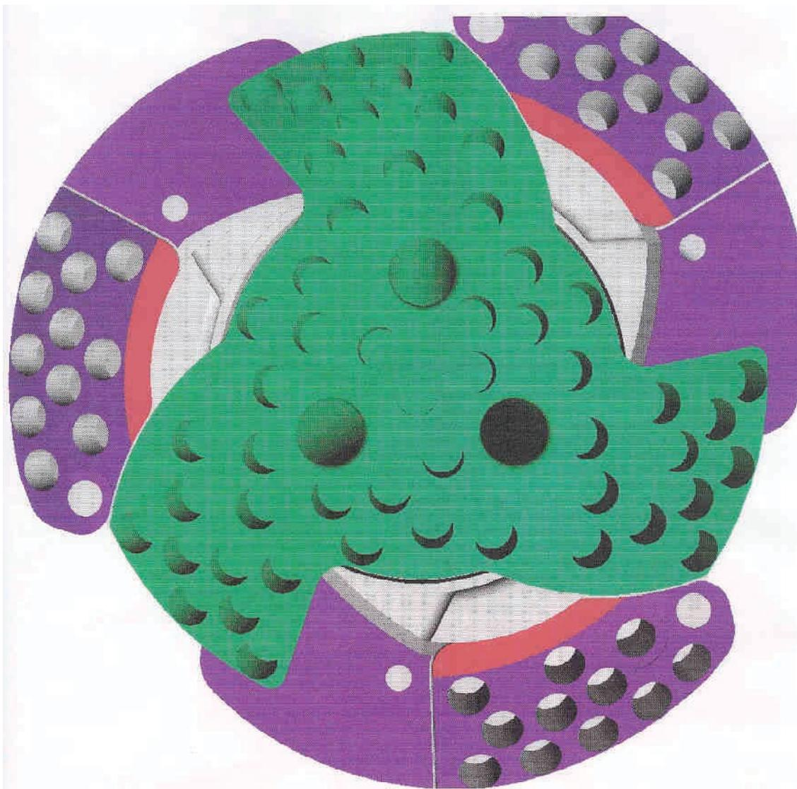
Figure F17. Dual cam underreamer bit in the closed position. Tungsten carbide inserts are not illustrated.
