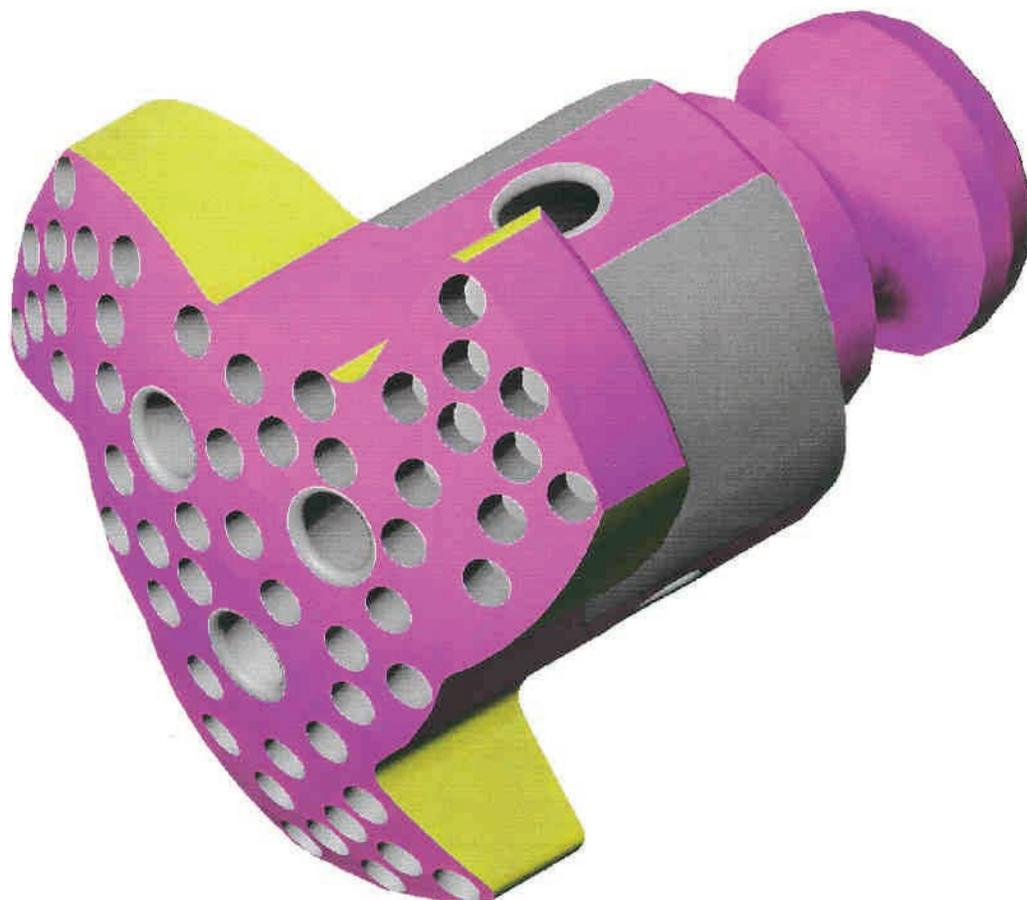
Figure F16. Dual cam underreamer bit in the open position. Tungsten carbide inserts are not illustrated.
