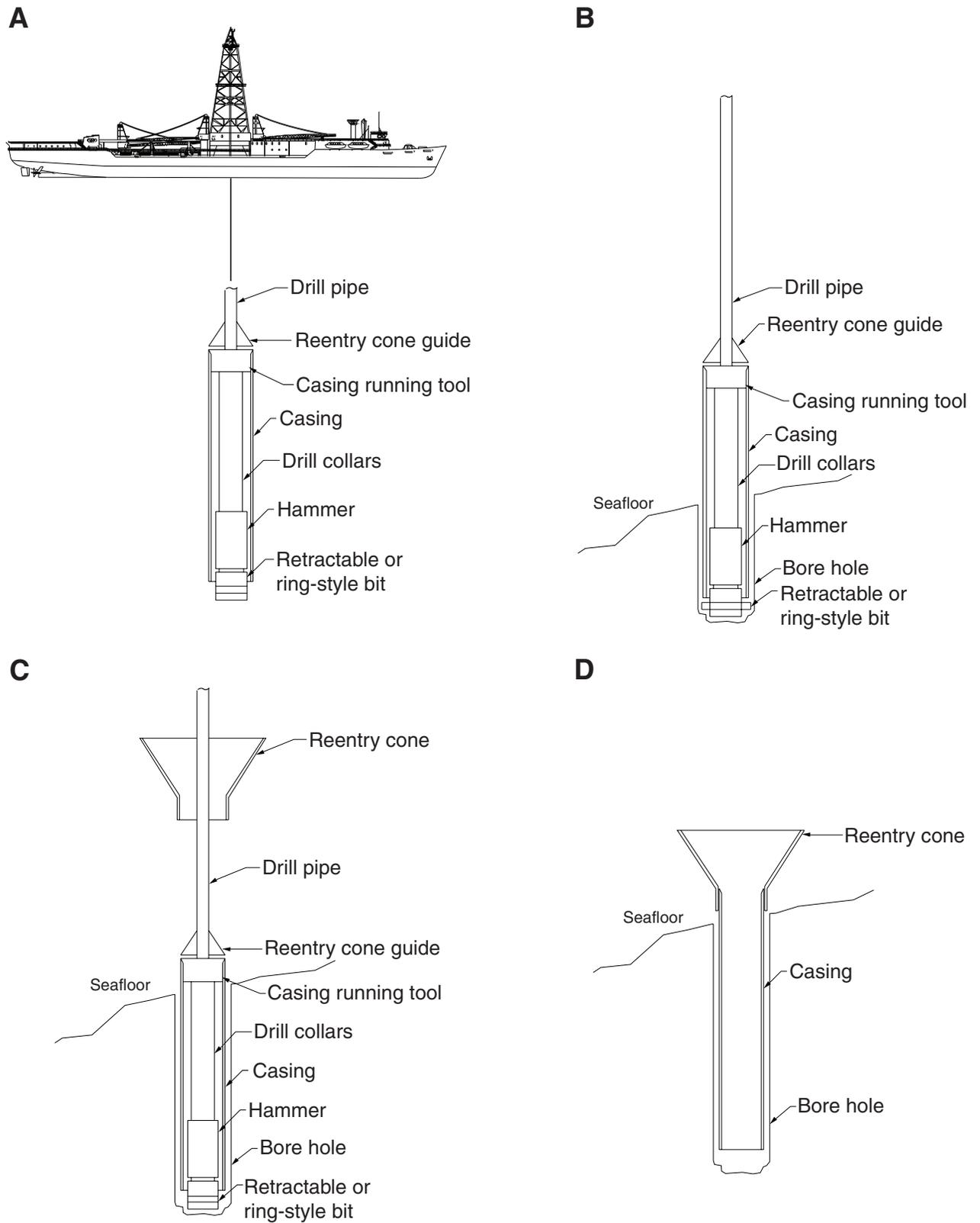
Figure F7. Running tool release after casing is drilled to depth. A. Reentry cone is deployed after casing is drilled in. B. Running tool is withdrawn after the dogs are released. Dashed lines show non-running tool components.
