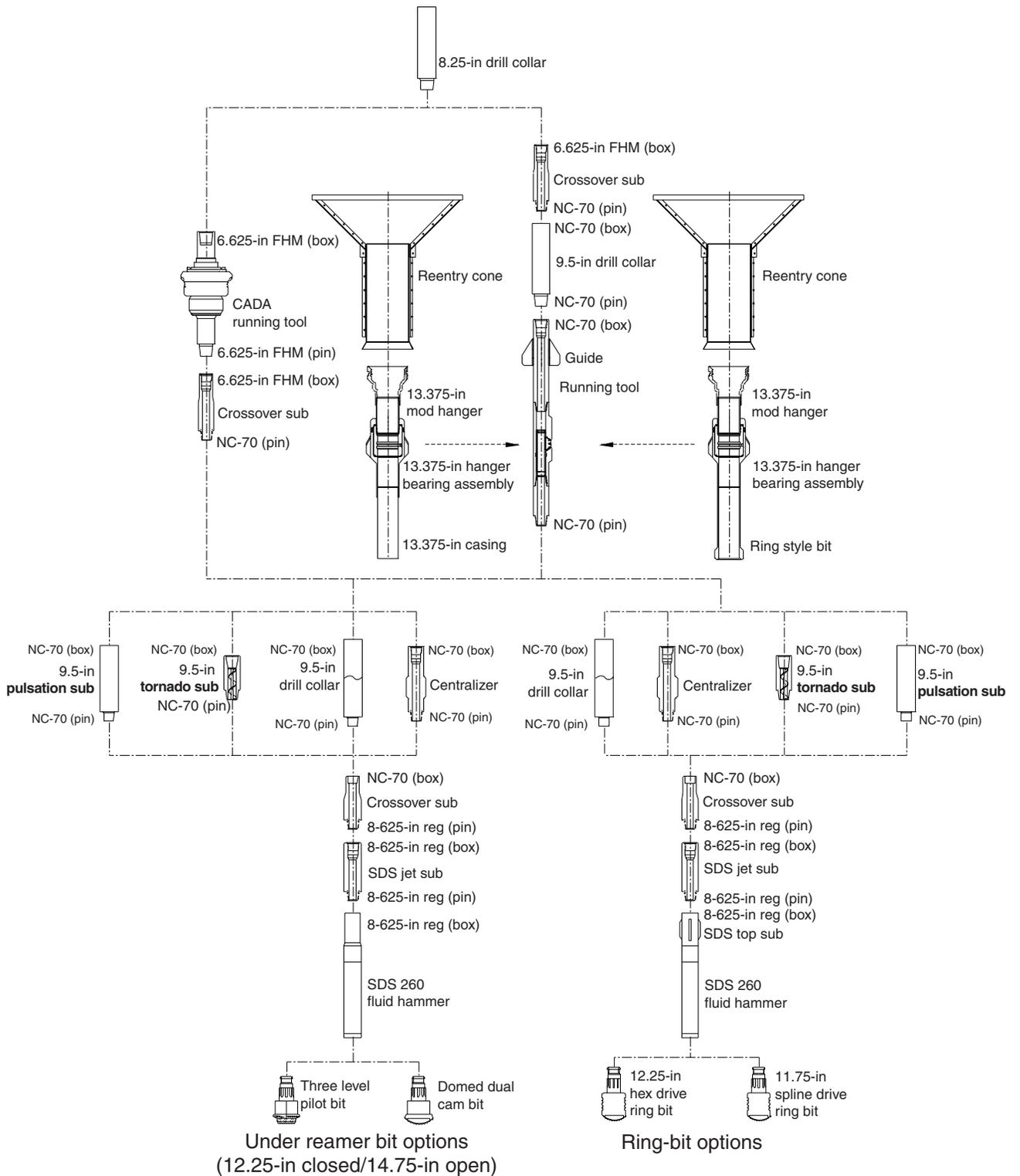
Figure F9. SDS Digger Tools 260 fluid hammer.
