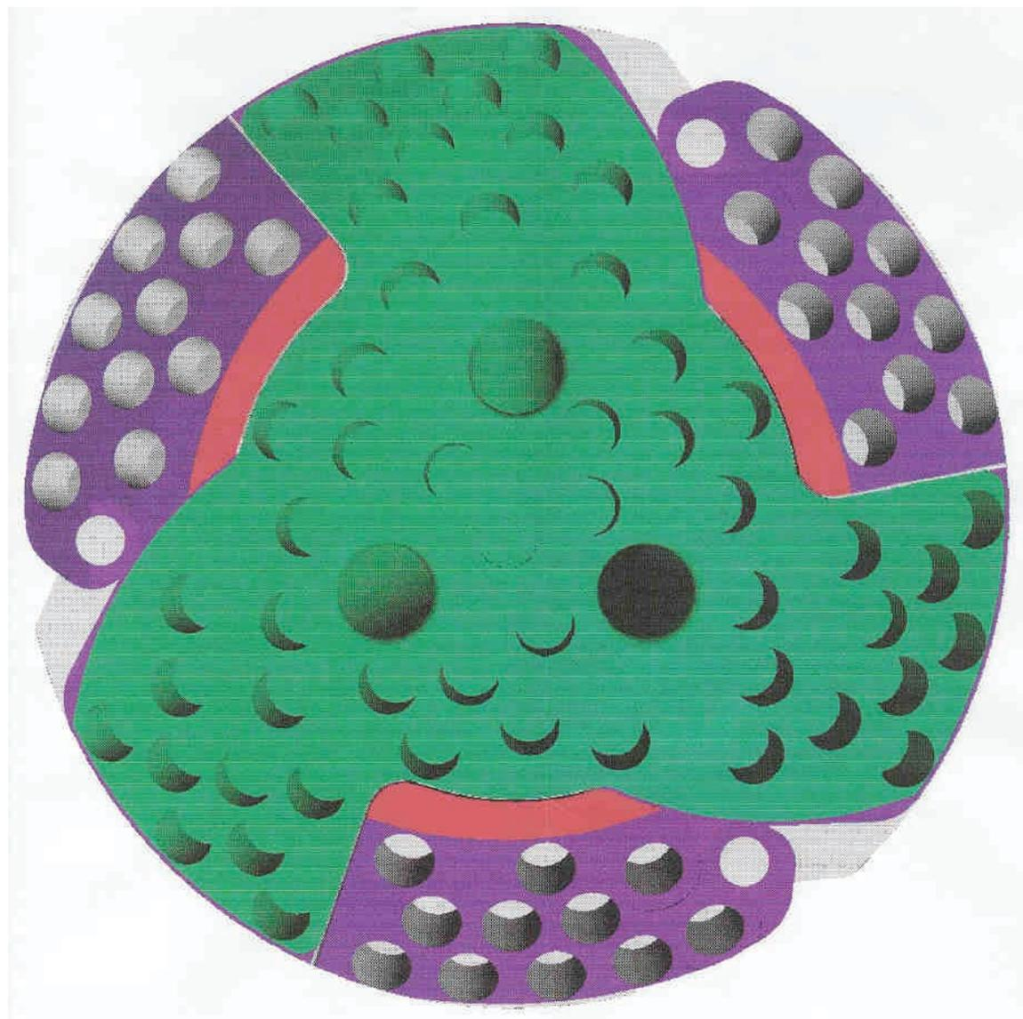
**Figure F18.** Three-level flat-face underreamer pilot bit. Tungsten carbide inserts are not illustrated.
