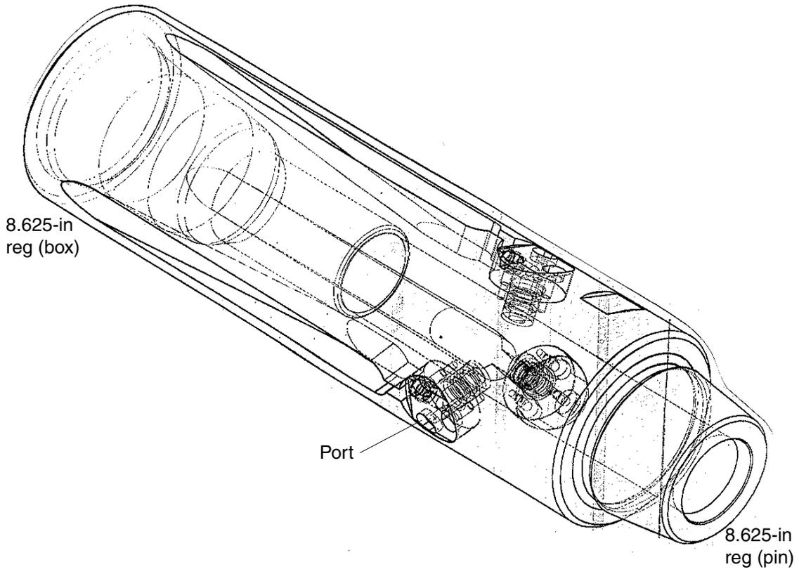
Figure F13. Profile of the dual cam underreamer bit. Tungsten carbide inserts are not illustrated.
