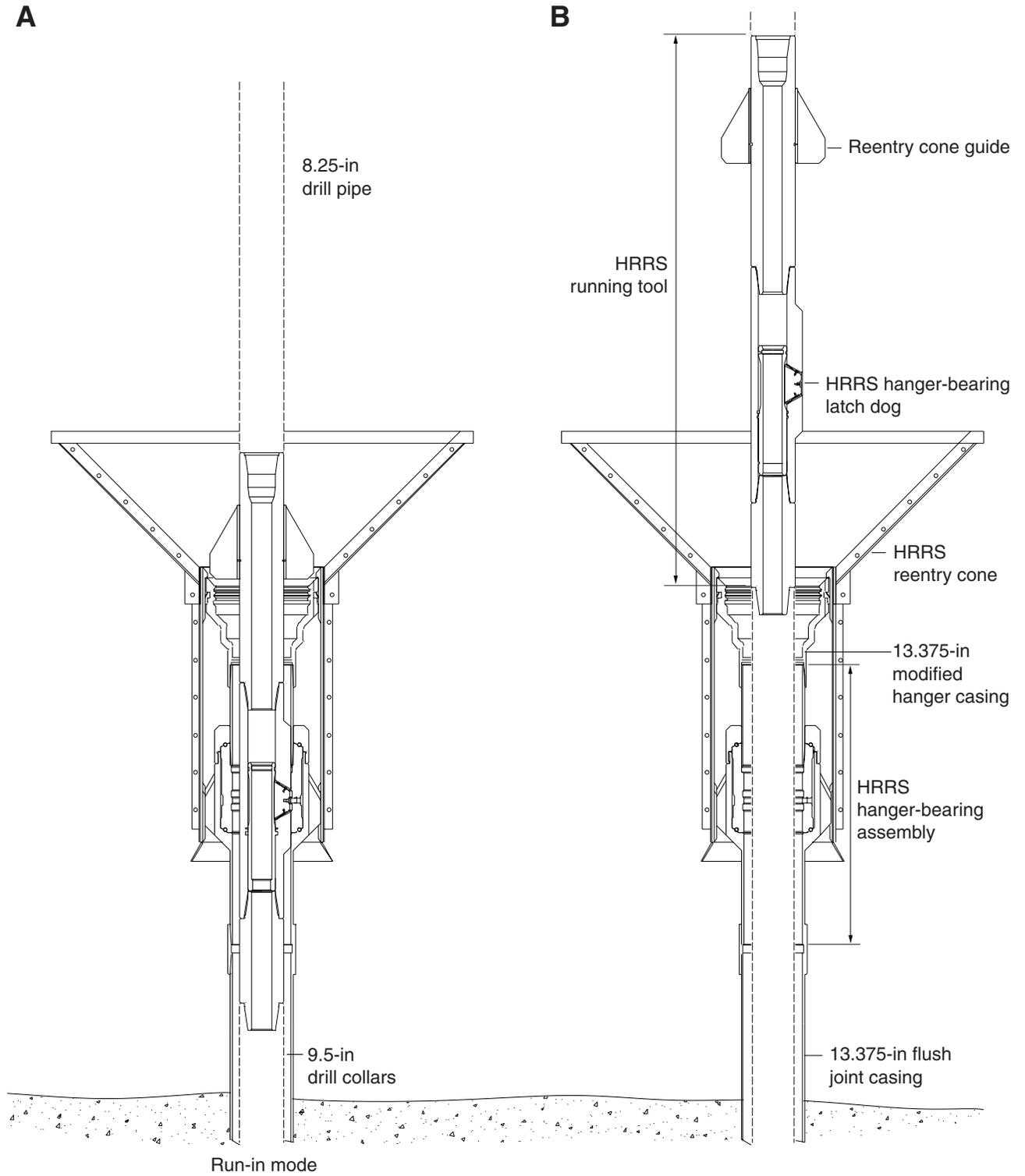
**Figure F8.** Hard-rock reentry system setup. NC-70 connections are cut on 9.5-in bodies. FHM = full hole modified, CADA = cam actuated drilling assembly.
