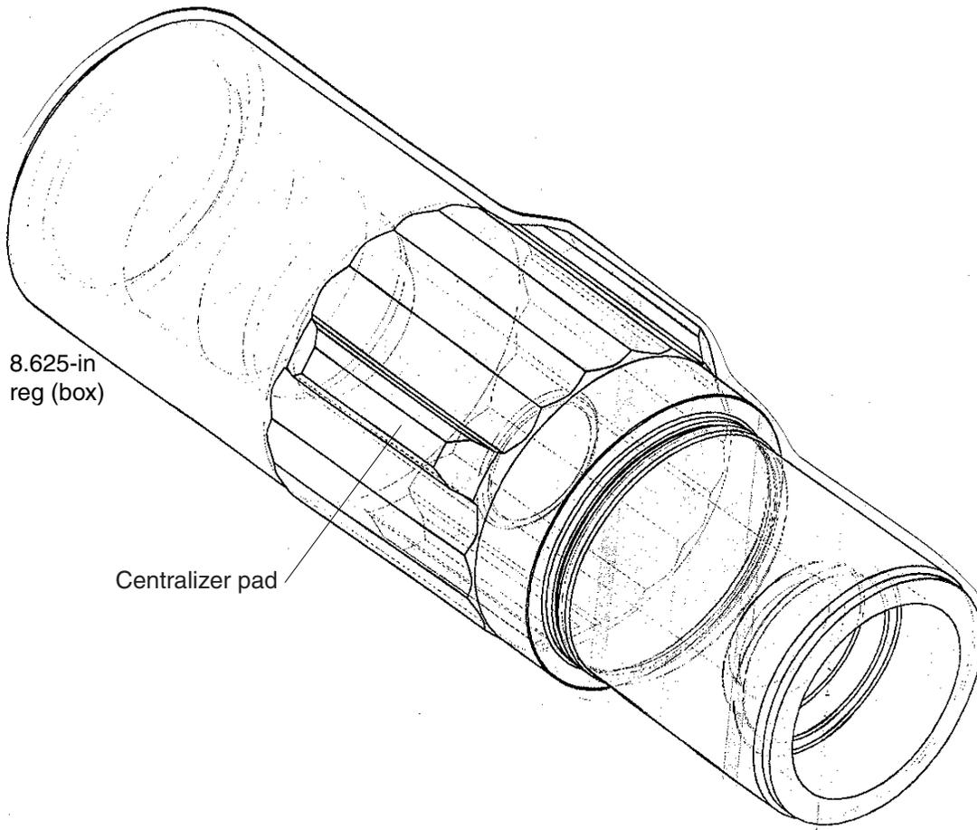
Figure F12. SDS modified jet sub (ODP style with 8.625-in reg connections).
