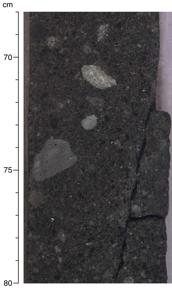
Figure F30. Interval 192-1184A-21R-6, 68–80 cm, showing lapilli tuff with basaltic clasts, altered black glass fragments, and accretionary and armored lapilli.
