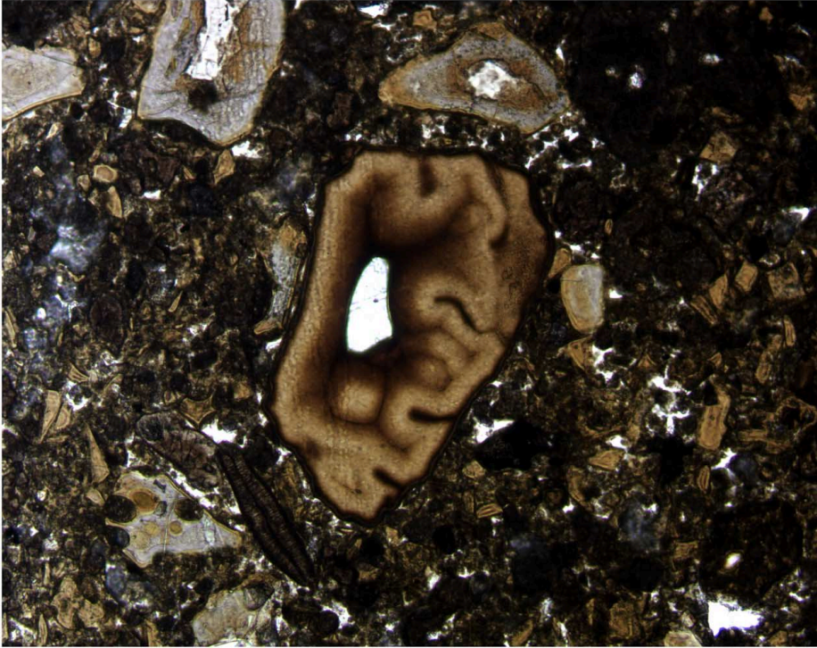
Figure F60. Altered glass fragment replaced by intricately zoned smectite at the rim and zeolite in the center in Sample 192-1184A-42R-1, 147–150 cm (field of view = 2.8 mm; photomicrograph ID#s 1184A_091 and 1184A_092). A. Plane-polarized light. B. Crossed polars.
