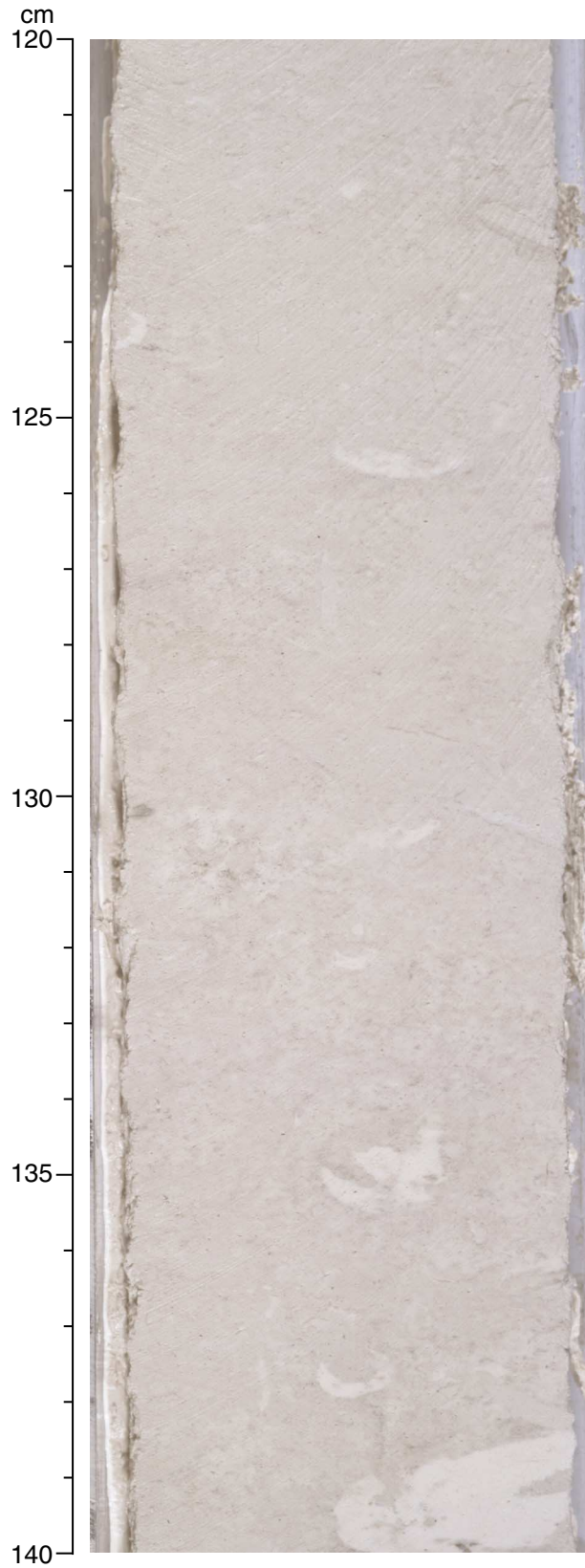
Figure F9. Typical light gray bioturbated chalk facies of Unit II (Eocene) from interval 192-1185A-6R-1, 120–140 cm.
