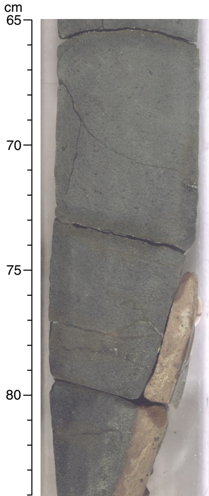
Figure F14. Interval 192-1185B-17R-1, 65–84 cm, showing pink, fine-grained limestone adjacent to fine-grained basalt. The limestone is interpreted as filling a fissure within the upper part of the massive flow of Unit 10.
