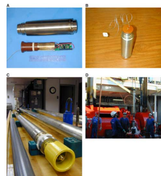
F14. Steps for assembling the core barrel temperature tool, p. 53.
