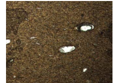
F3. Fresh rhyodacite with about equal proportions of volcanic glass and fine microcrystalline plagioclase needles, p. 16.
