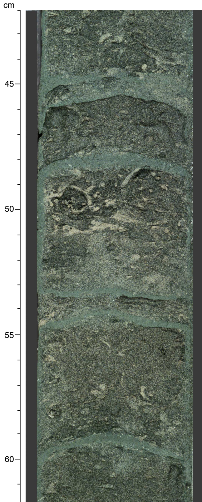
Figure F9. Close-up photograph of Sample 194-1195B-50X-1, 42–62 cm (468.12 mbsf; Unit IV), showing medium-sized, well-sorted greenish gray sand with glauconite. Chondrites appear as common white burrows.
