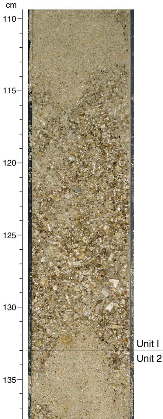
Figure F5. Close-up photograph of interval 194-1195A-5H-1, 110–138 cm, showing a coarse and poorly sorted skeletal-rich floatstone with light brown phosphatized lithoclasts, interlayered with foraminiferal grainstone. The base of the floatstone layer at 34.5 mbsf represents the boundary between Units I and II at Site 1195A.
