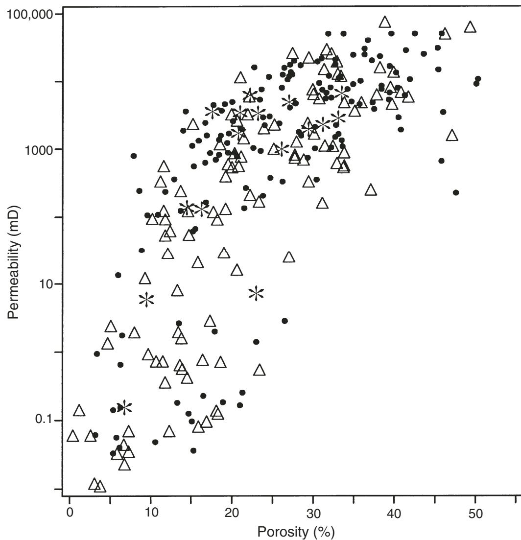
**Figure F5.** Klinkenberg-corrected gas permeability vs. porosity for plugs from Site 1199. Solid circles = horizontal plugs (EHRE samples), triangles = vertical plugs (BRAG samples), stars = whole-core (EHWR samples).
