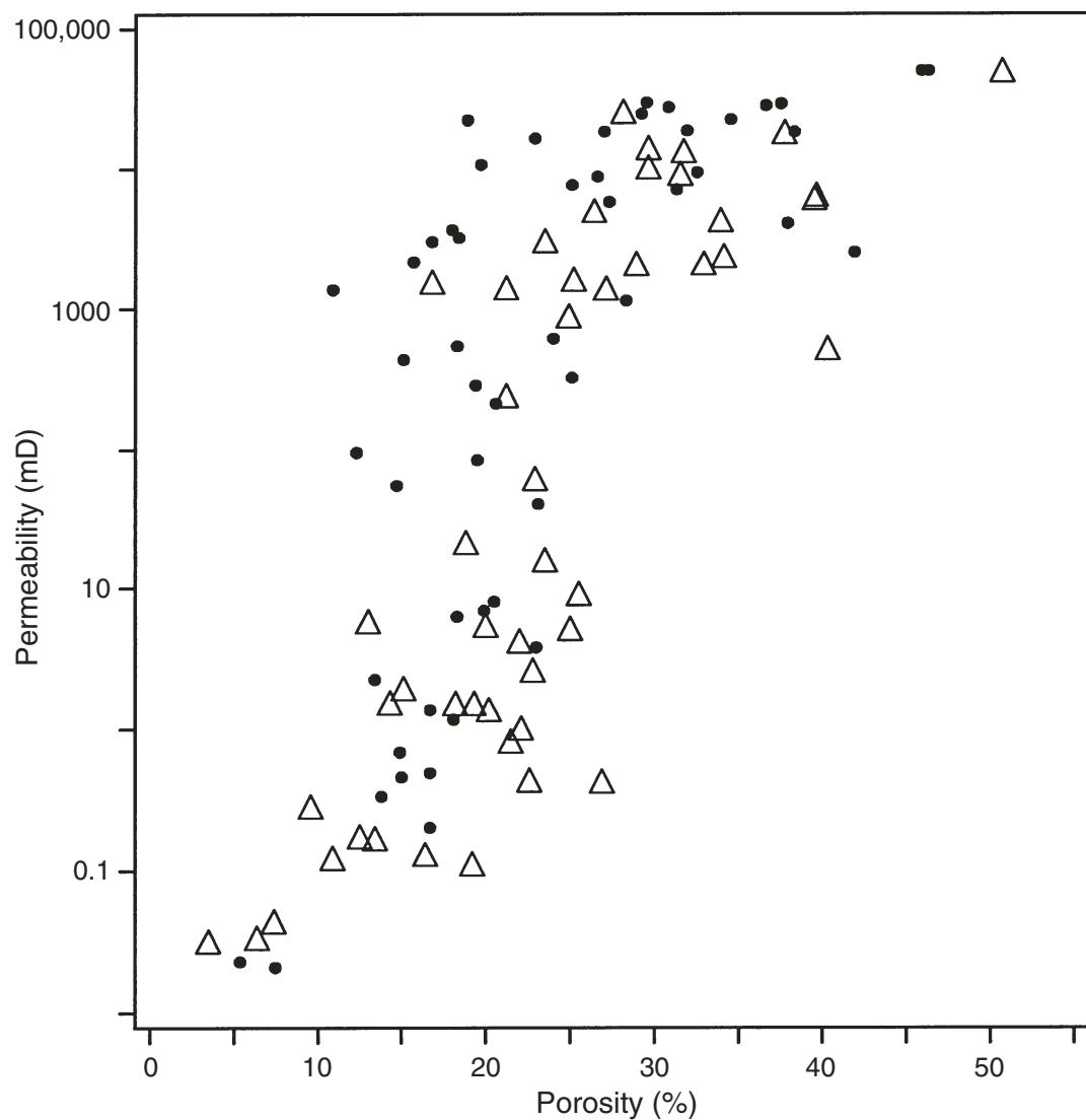
**Figure F4.** Klinkenberg-corrected gas permeability vs. porosity for plugs from Site 1196. Solid circles = horizontal plugs (EHRE samples), triangles = vertical plugs (BRAG samples), stars = whole-core (EHWR samples).
