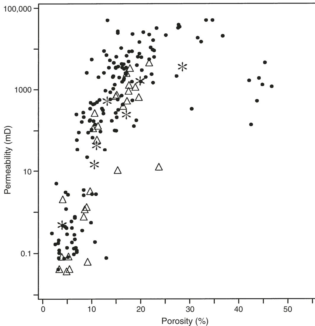
Figure F6. Permeability vs. porosity of samples from slope sites. Open circles = Site 1193, solid circles = Site 1194, shaded squares = Site 1195, open squares = Site 1197, stars = Site 1198.
