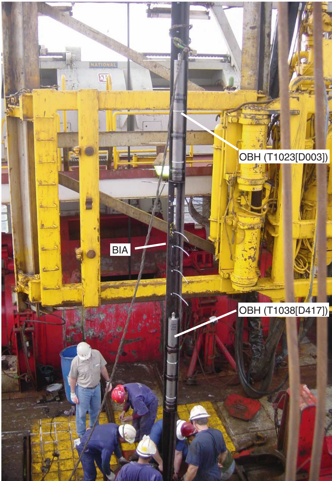
Figure F17. Borehole seismometer instrument package deployed in Hole 1201D. BIA = borehole instrument assembly, OBH = ocean borehole seismometer.
