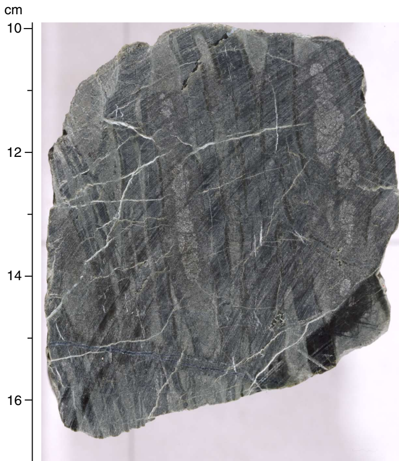
Figure F28. Color photograph of variably serpentinized dunite forming dark bands where completely altered. The banding of the sample is crosscut by later white chrysotile veins (interval 195-1200A-13R-1, 10–17 cm).
