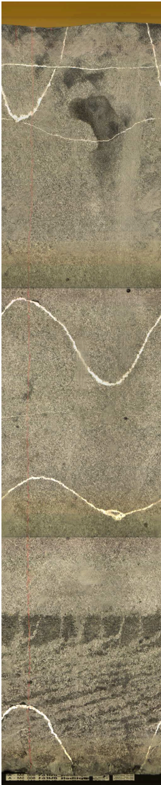
Figure F53. Well-defined dipping veins showing sinusoidal pattern in the DMT image of Site 1203 basalt.
