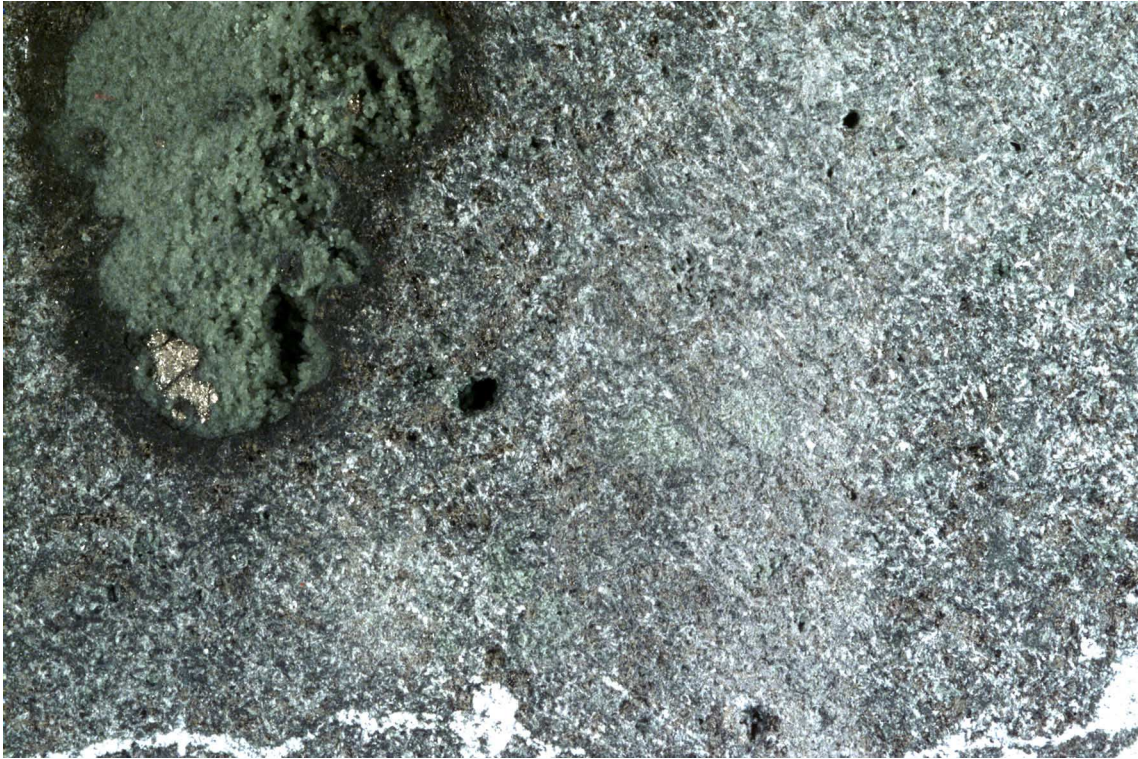
Figure F35. Close-up photograph of a megavesicle filled with saponite and pyrite (interval 197-1204A-10R-3, 98–100 cm). Note: the photograph was taken on the working half of the core.
