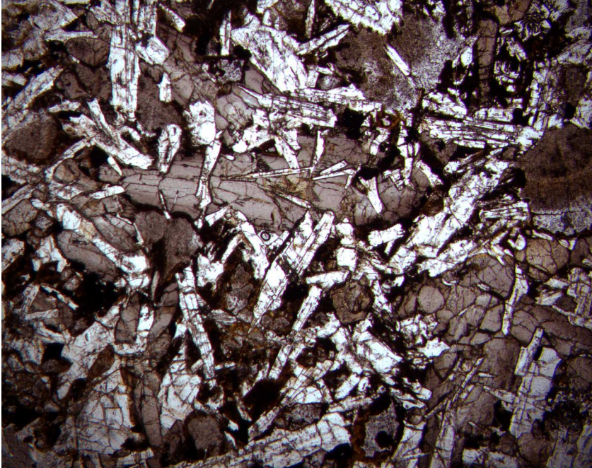
Figure F15. Photomicrograph of subophitic texture showing clinopyroxene with a pink hue partially enclosing plagioclase laths (Sample 197-1204B-7R-3, 140-142 cm ) (plane-polarized light; field of view = 5 mm; photomicrograph 1204B-131).
