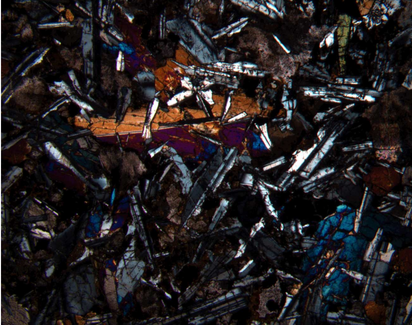
Figure F14. Photomicrograph of subophitic texture showing clinopyroxene partially enclosing plagioclase laths (Sample 197-1204B-7R-3, 140–142 cm) (cross-polarized light; field of view = 5 mm; photomicrograph 1204B-130).
