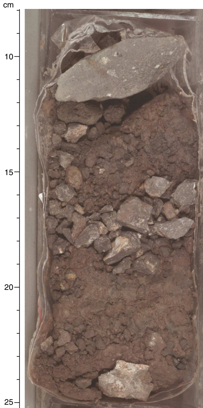
Figure F8. Photograph showing red clay soil of Unit 7 and relatively unweathered basalt units immediately above (to the left) and below (interval 197-1205A-19R-4, 8–25 cm).
