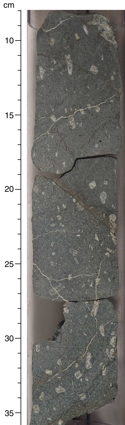
Figure F9. Photograph showing highly plagioclase-phyric alkali basalt of basement Unit 1 (interval 197-1205A-6R-1, 8–36 cm).
