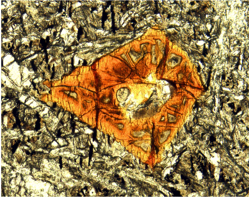
Figure F9. Photomicrograph of euhedral olivine altered to iddingsite in Unit 4 (Sample 197-1206A-8R-2 [Piece 1, 2-3 cm]) (plane-polarized light; field of view = 0.625 mm; photomicrograph 1206A-317).
