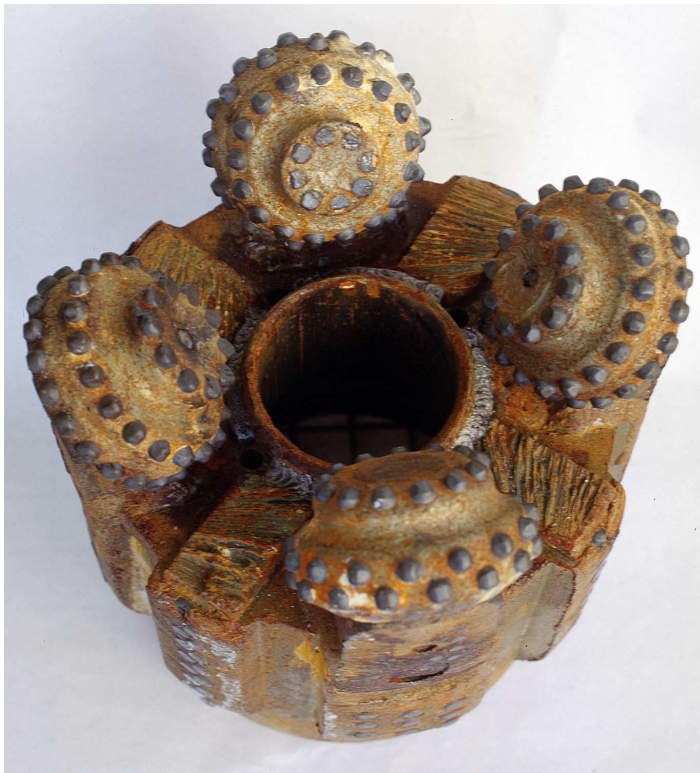
Figure F5. Photographs of (A) damaged bit and (B) locable float valve. Note the broken hinge pin and chert fragments inside the LFV housing.
