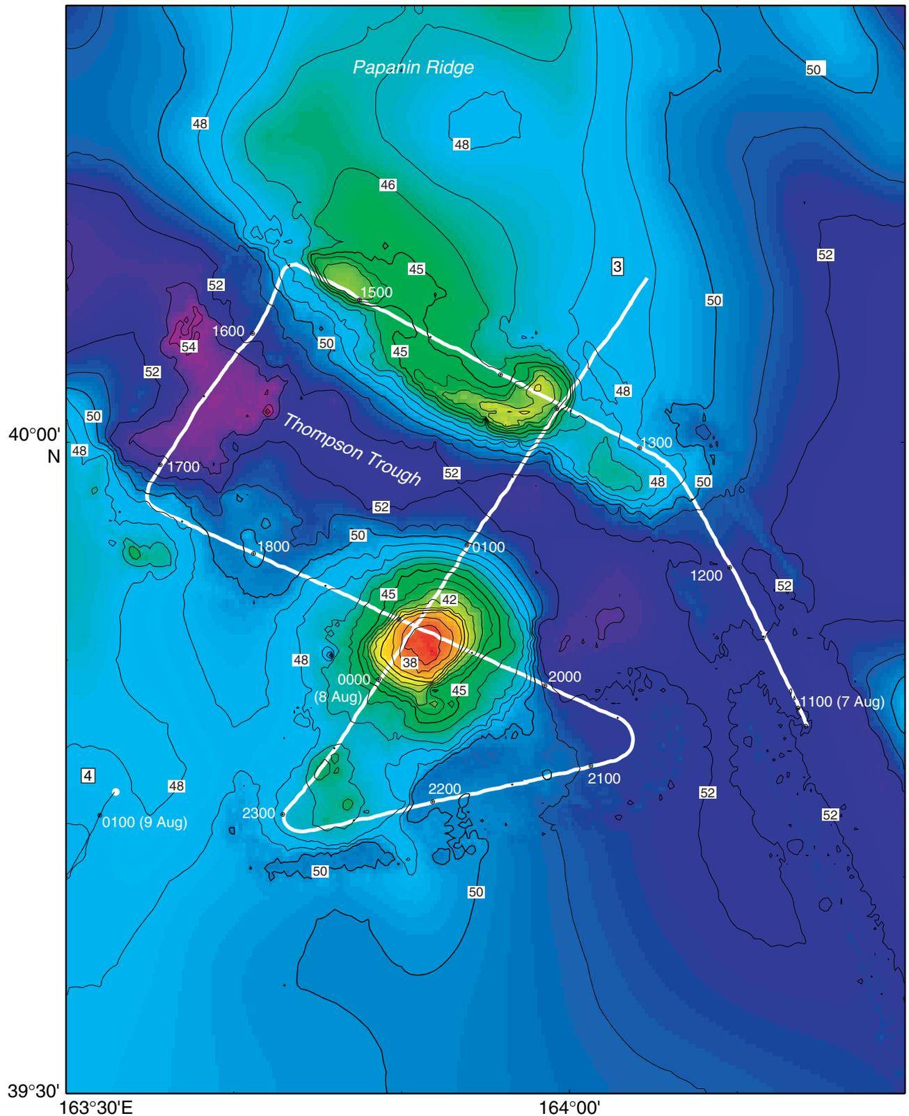
Figure F6. Seismic data acquisition geometry, sources, and receivers used on the *Thomas Thompson* cruise TN037 over Shatsky Rise. GI = generator injector, GPS = Global Positioning System.
