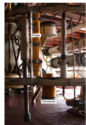
F18. The 4.252-kHz transducer, pinger batteries, and electronics on the VIT frame, p. 61.
