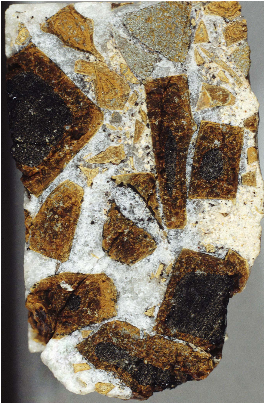
Figure F35. Scanned image of flow-top hyaloclastite from Unit 2 cemented by calcite (Sample 200-1224F-6R-1 [Piece 6, 29–33 cm]). Fresh glass is very dark gray; altered glass is gray; orange is palagonitized glass. Calcite is white to light gray.
