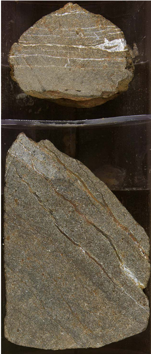
Figure F36. Close-up photograph of an array of subparallel oblique fractures lined with iron oxyhydroxides and calcite (Sample 200-1224F-14R-1 [Pieces 7–8, 62.5–76.5 cm]; Unit 3). Most of the rock is at least partially stained uniformly with iron oxyhydroxides, which also line the three larger fractures in lower Piece 8. Calcite later lined the same fractures, as well as the fractures in Piece 7.
