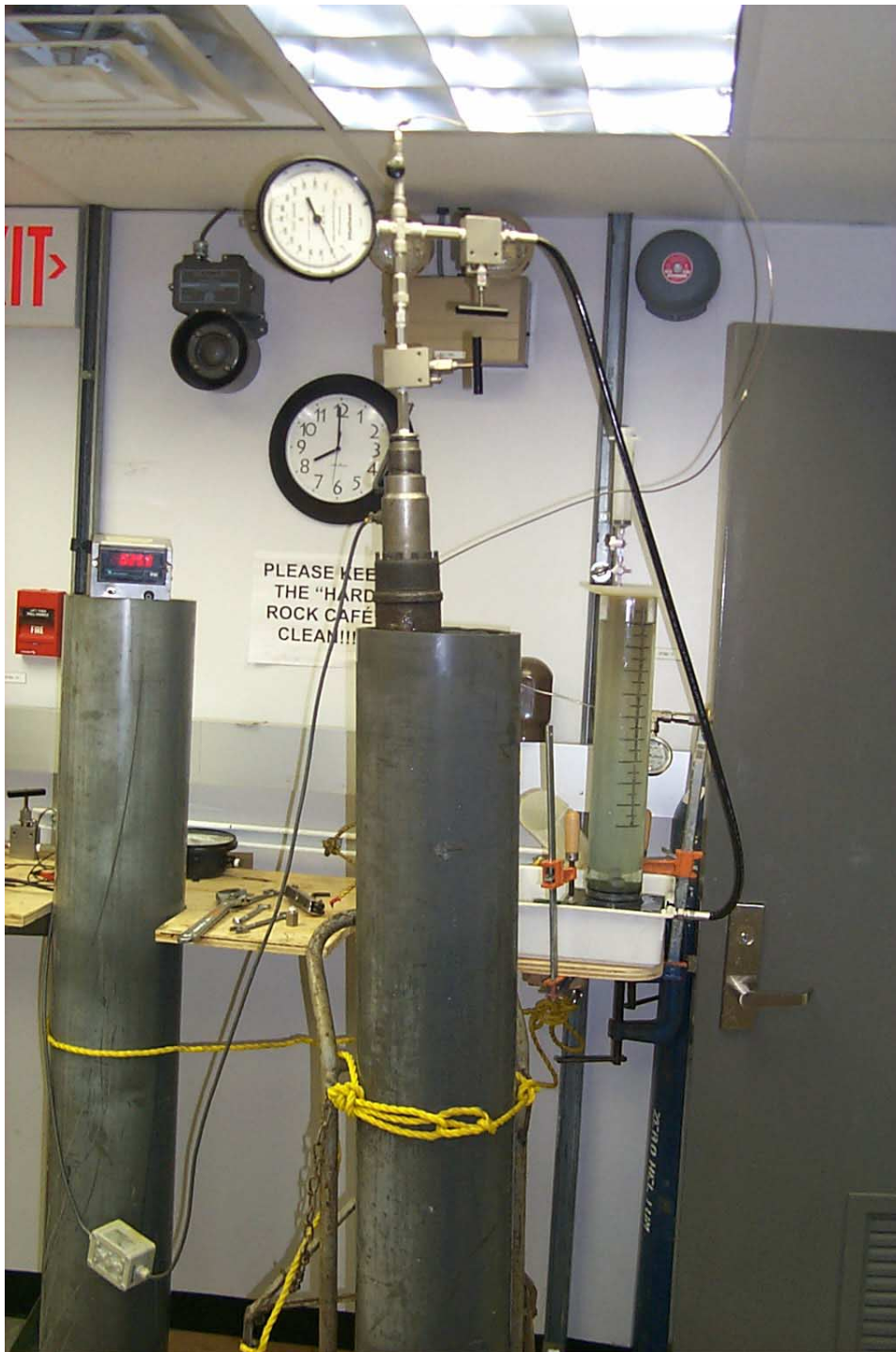
Figure F3. Photograph showing the gas manifold system and degassing of the PCS in the laboratory during Leg 201.
