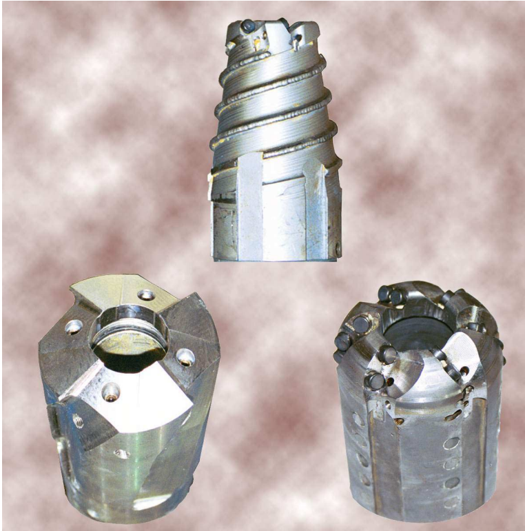
Figure F2. Photograph showing new cutting shoes used during PCS deployments. Left: Christensen auger shoe with carbide cutters. Middle: Rock Bit International (RBI) tapered auger shoe with PDC cutters. Right: RBI standard PDC cutting shoe.
