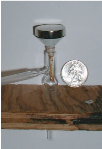
Figure F1. Magnetized needle used for extraction of <math><7\text{-}\mu\text{m}</math> size fraction. Coin diameter = 24 mm.
