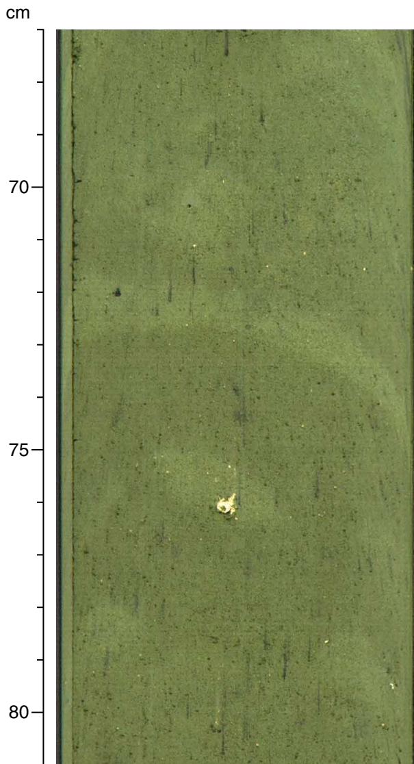
Figure F16. Close-up photograph of Unit I major lithology showing homogeneous grayish olive-green color, burrows, and spicule aggregates (interval 202-1242B-2H-6, 67–81 cm).
