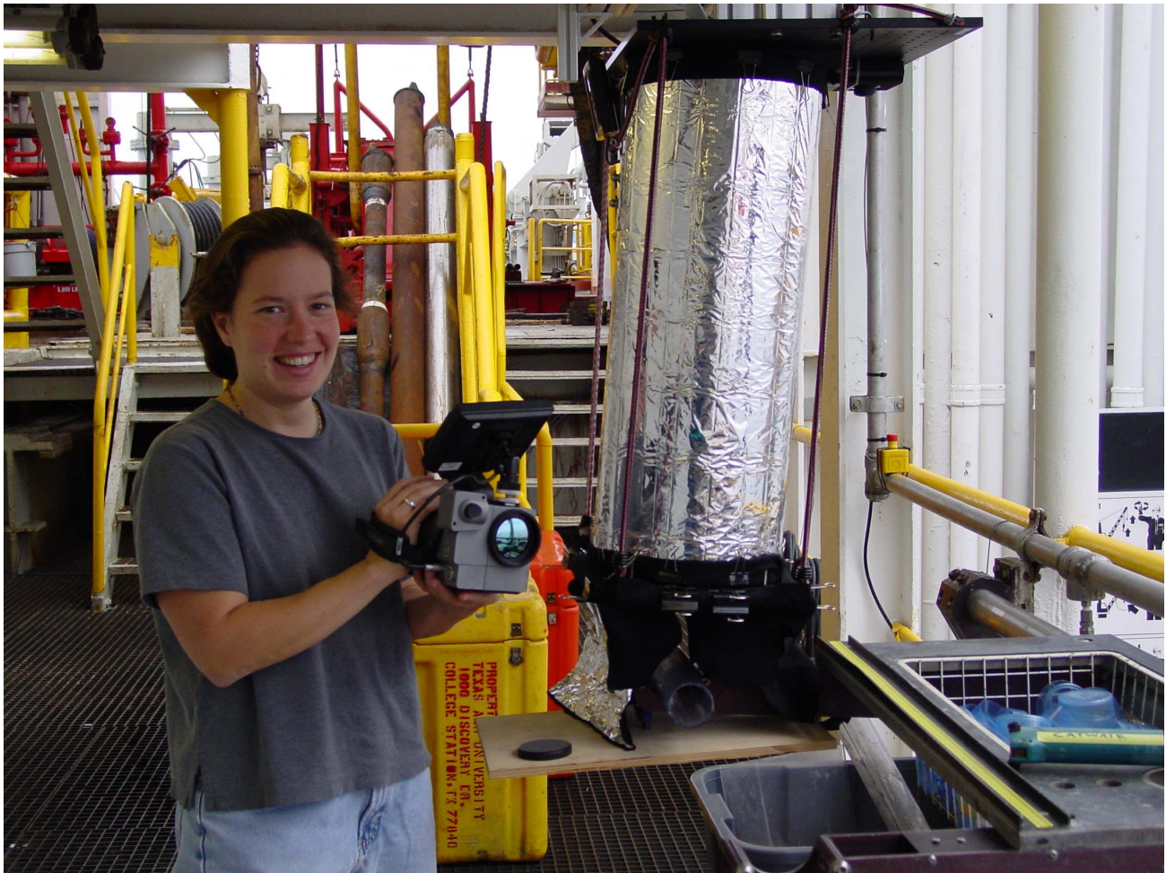
Figure F10. Sedimentologist Jill Weinberger holds a FLIR SC-2000 camera used for IR thermal imaging during Leg 204. The camera was mounted on a track inside a tubular structure designed to reduce extraneous infrared reflections.
