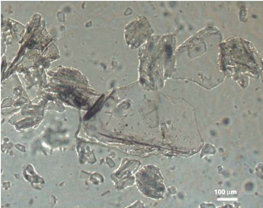
Figure F14. Photomicrograph of sand-sized volcanic glass within the Horizon A volcanic glass-rich sediment and ash sequence in lithostratigraphic Subunit IIIA (Sample 204-1245B-21X-4, 36 cm [180.86 mbsf]) (200×).
