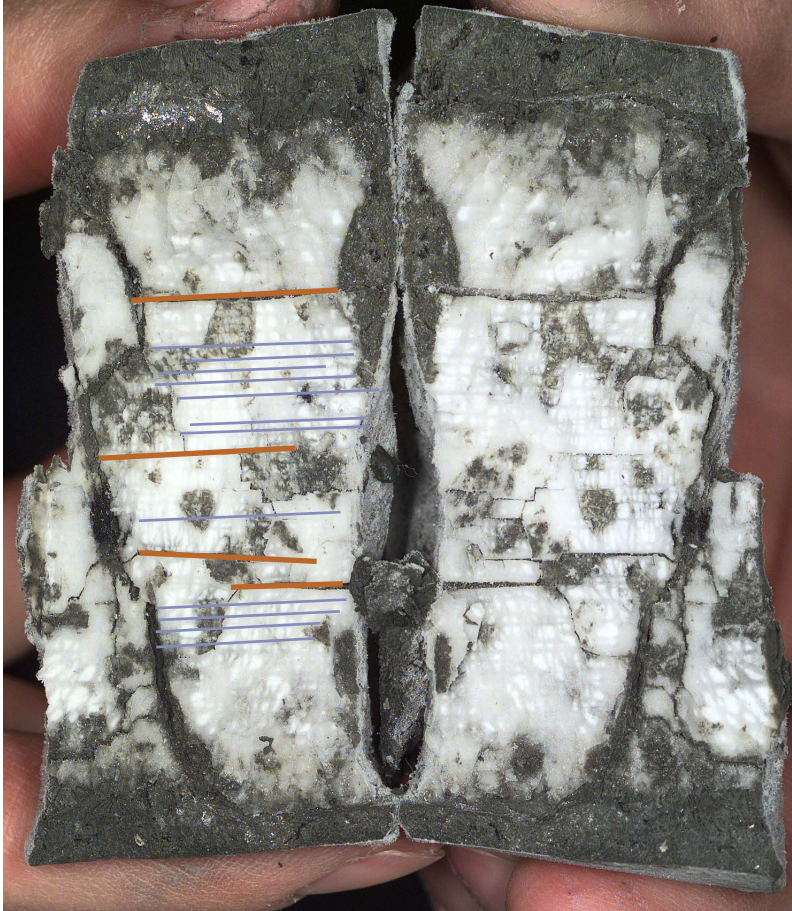
Figure F10. Close-up photograph of Sample 204-1249F-8H-2, 117–127 cm (diameter of whole-round sample is 6.6 cm). Blue lines = closely spaced cleavage planes. Red lines = planes with an offset.
