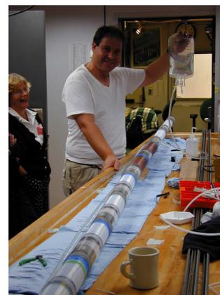
F6. Sampling section of the intake probe, Hole 1255A, p. 20.
