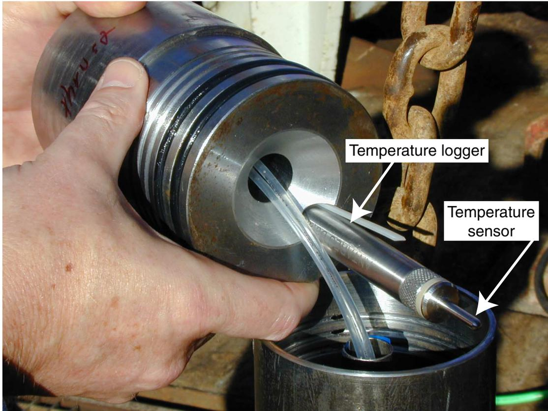
Figure F10. Close-up photograph of the data logger bay of the CORK-II head.
