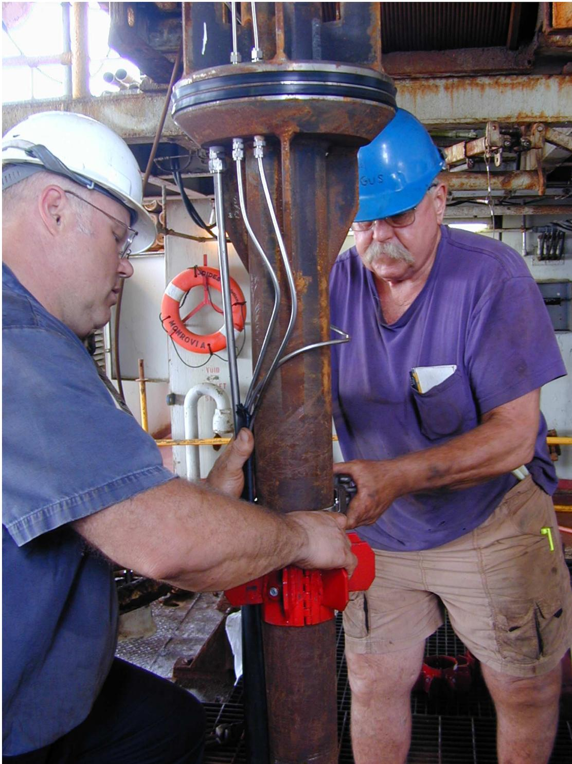
Figure F20. CORK-II head bay with plumbing and valves.
