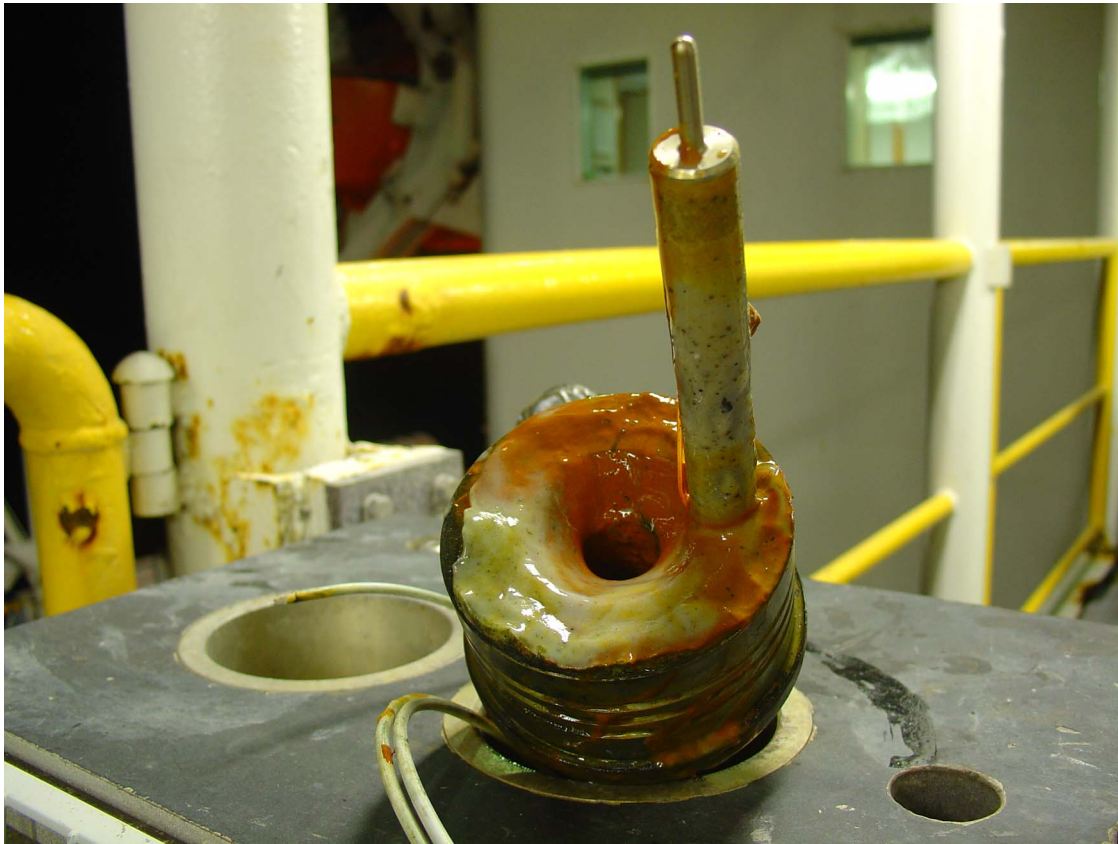
Figure F5. MTL in Hole 1253A after recovery from 2-yr deployment.
