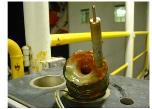
F5. Recovered MTL after 2-yr deployment, p. 13.
