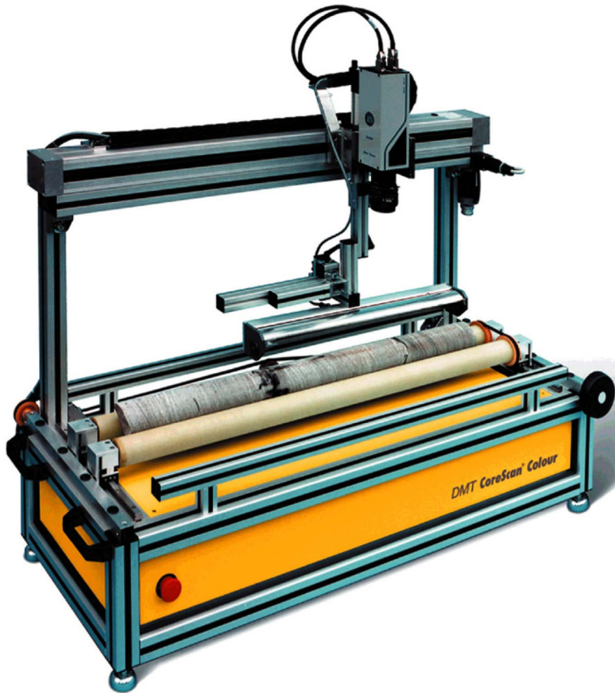
Figure F18. Photograph of the DMT Digital Color CoreScan system used during Leg 206.
