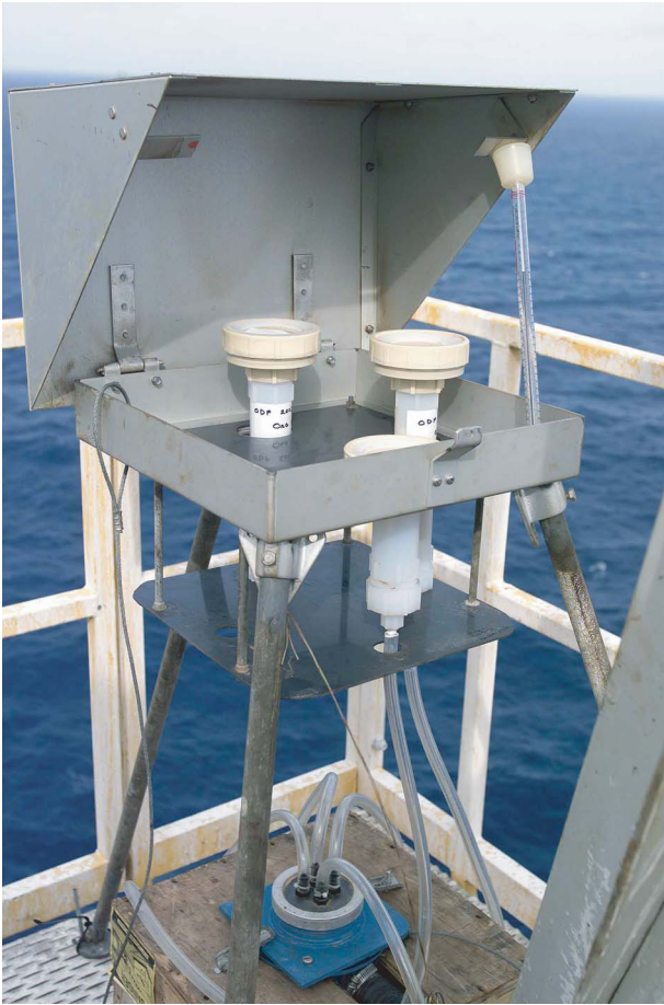
Figure F14. Air sampler for analysis of metals and organic pollutants.
