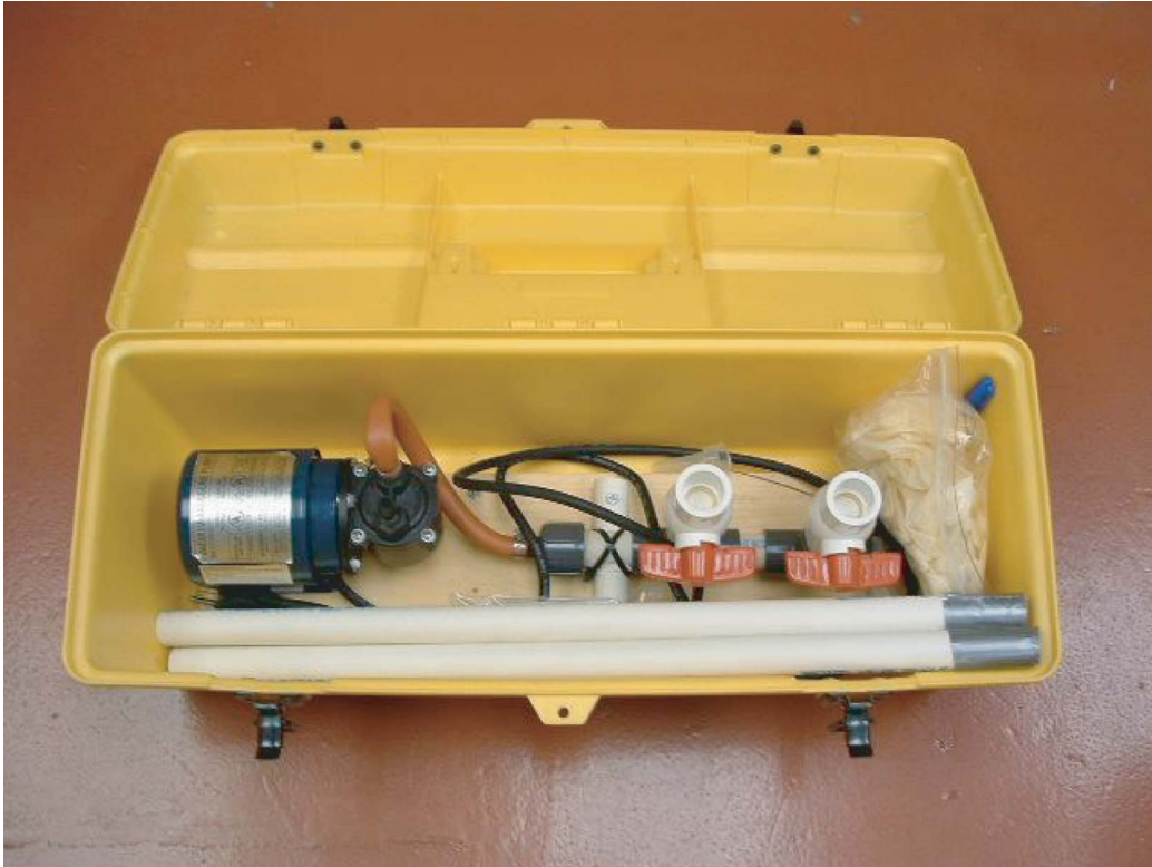
Figure F12. Portable membrane filtration apparatus for atmospheric microbiology culture-based studies.
