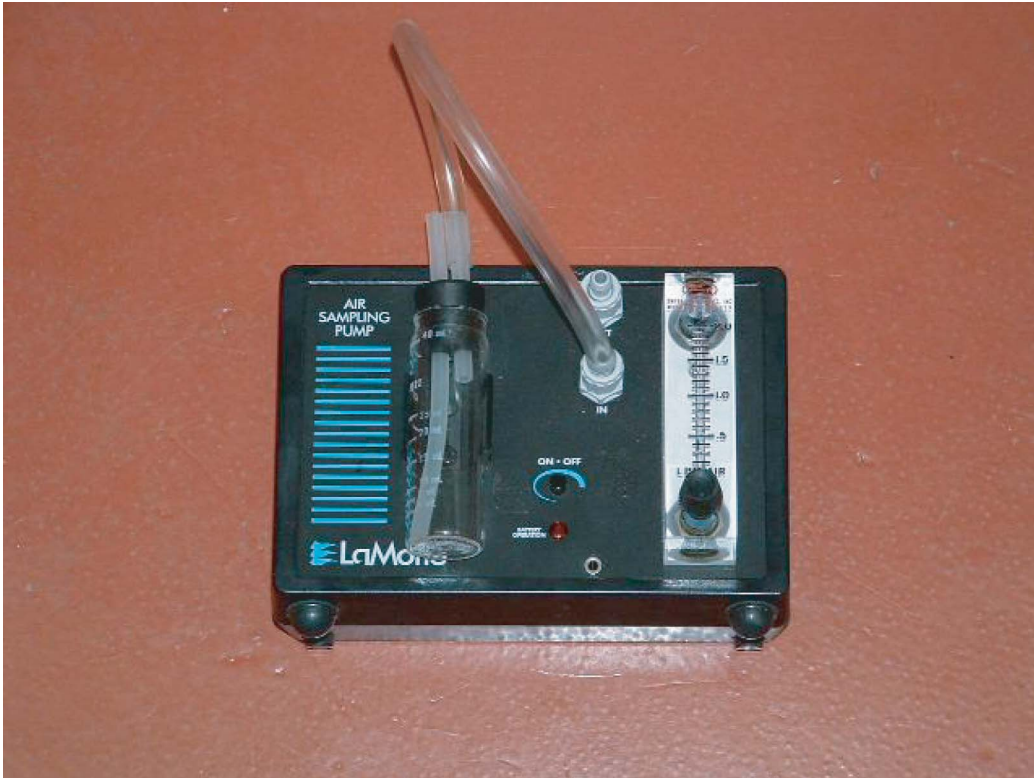
Figure F13. Portable liquid impinger for atmospheric collection of microorganisms for molecular and transmission electron microscopy analysis.
